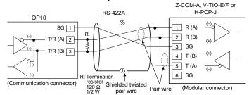
If communication error repeats frequently because of operating environment and/or communication distance, try to connect a terminal resistor also on the controller side. Refer to the instruction manual of the relevant controller for details of the terminal resistor on the controller side.
