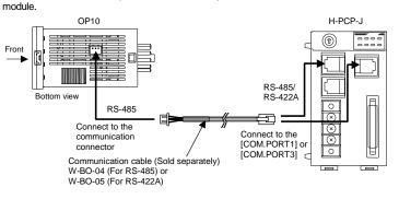
Up to 16 H-PCP-J modules can be connected (however, up to 99 channels).
