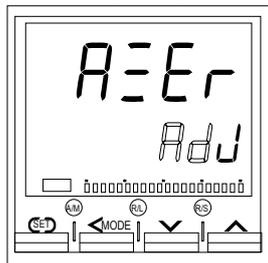
Adjust the zero point of the measured value (PV1) of Input 1.
