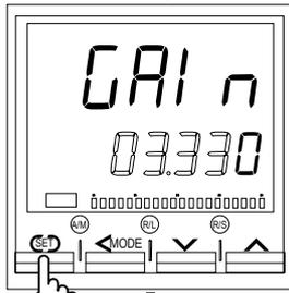
Use to set the gain of the pressure sensor input.
