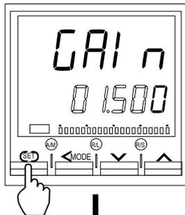
Use to set the gain of the pressure sensor input.
