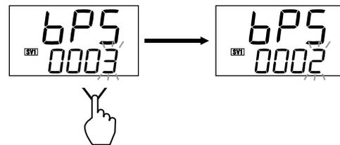
Press the SET key to store the new set value. The display goes to the data bit configuration.
