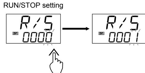
Press the SET key to store the new set value. The display goes to the function block 00 (F00.). The STOP lamp lights up and the controller enters the STOP state.
