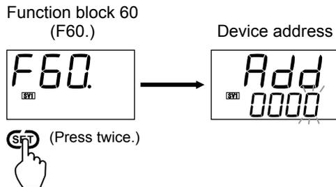
Set the device address (slave address).
