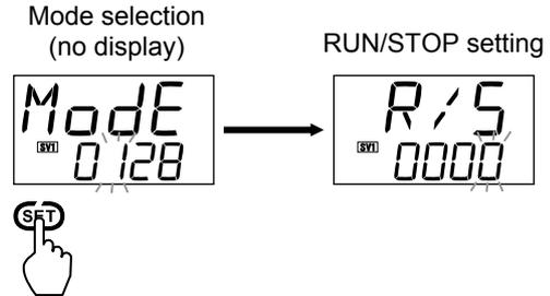
When “128” is set, display of the parameters from function block 21 (F21.) to function block 91 (F91.) is enabled.
