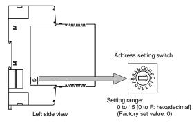
Up to four COM-JE units can be connected to a PLC communication port. Therefore the unit address uses the four COM-JE units as a group. Use consecutive numbers in any one of four groups in the following table as address.
