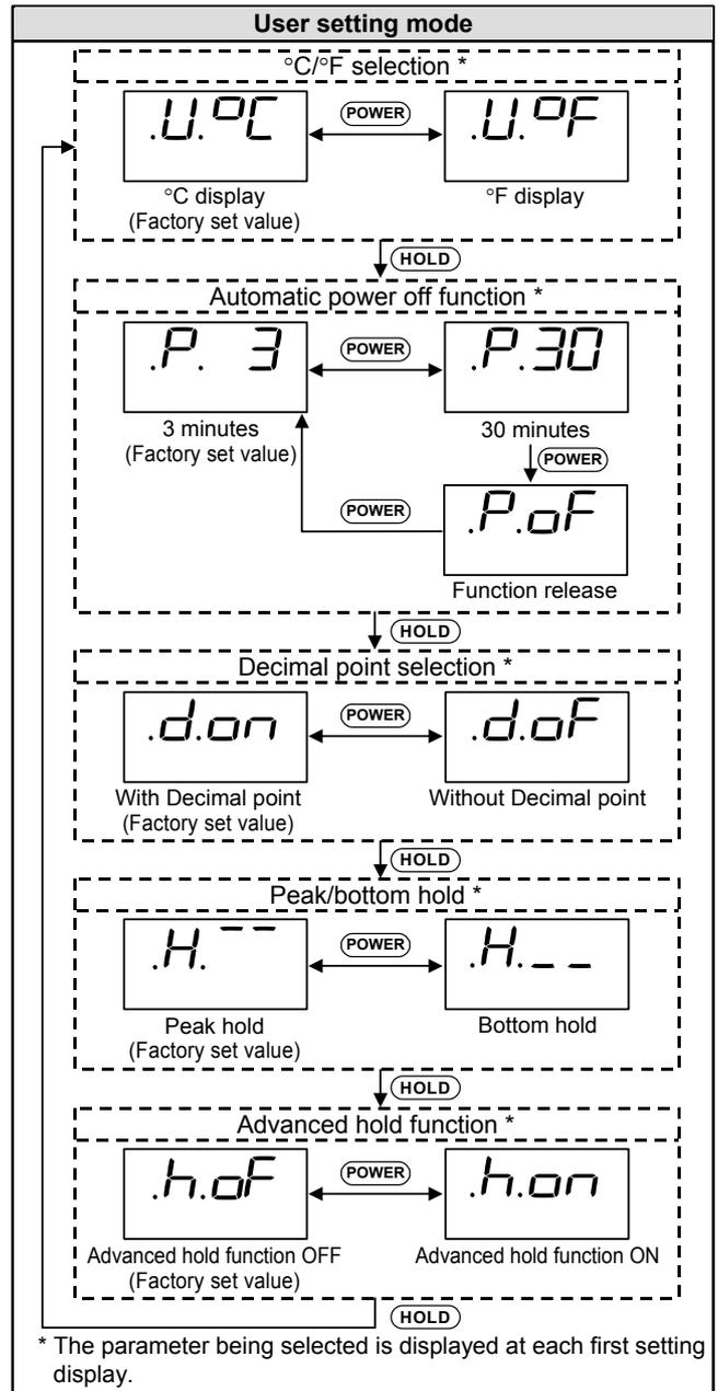
\* The parameter being selected is displayed at each first setting display.
