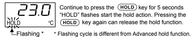
The peak/bottom hold function can be selected in “Peak/bottom hold” screen of User setting mode. (Factory set value: Peak hold)
