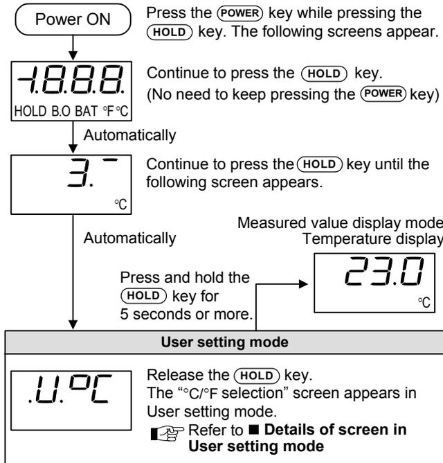
It is impossible to enter User setting mode from Measured value display mode.
