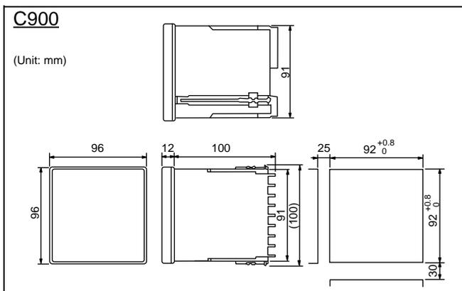
Panel thickness: 1 to 5 mm or 5 to 9 mm (C100)
