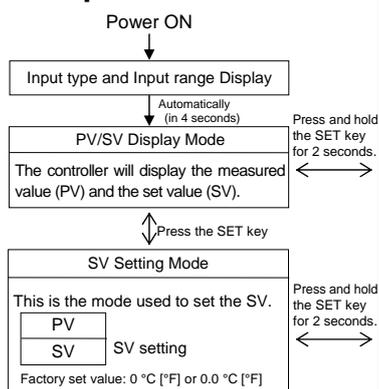
This instrument returns to the PV/SV display mode if no key operation is performed for more than one minute.
