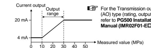
For the Transmission output (AO) type (rating, output range), refer to **PG500 Installation Manual (IMR02F01-ED)**.
