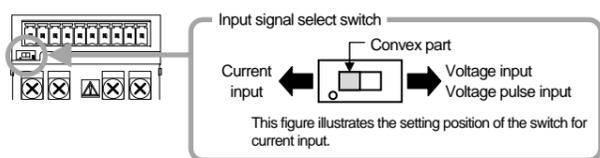
This figure illustrates the setting position of the switch for current input.
