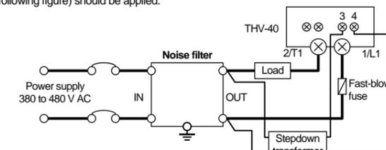
The noise filter specified: SOSHIN ELECTRIC CO., LTD.
