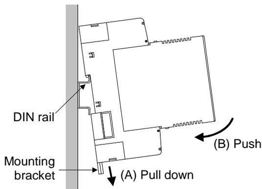
2. Slide the mounting bracket up to secure the module to the DIN rail.
