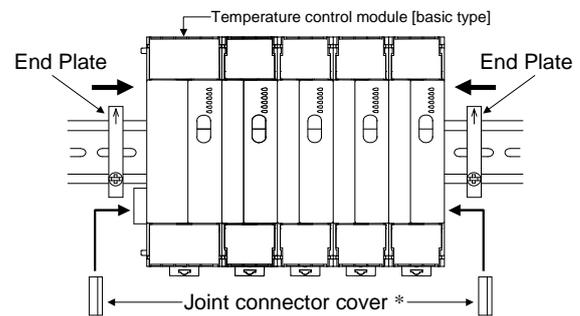
\* For the conservation of the contact of connector, install a joint connector cover in module of both ends.
