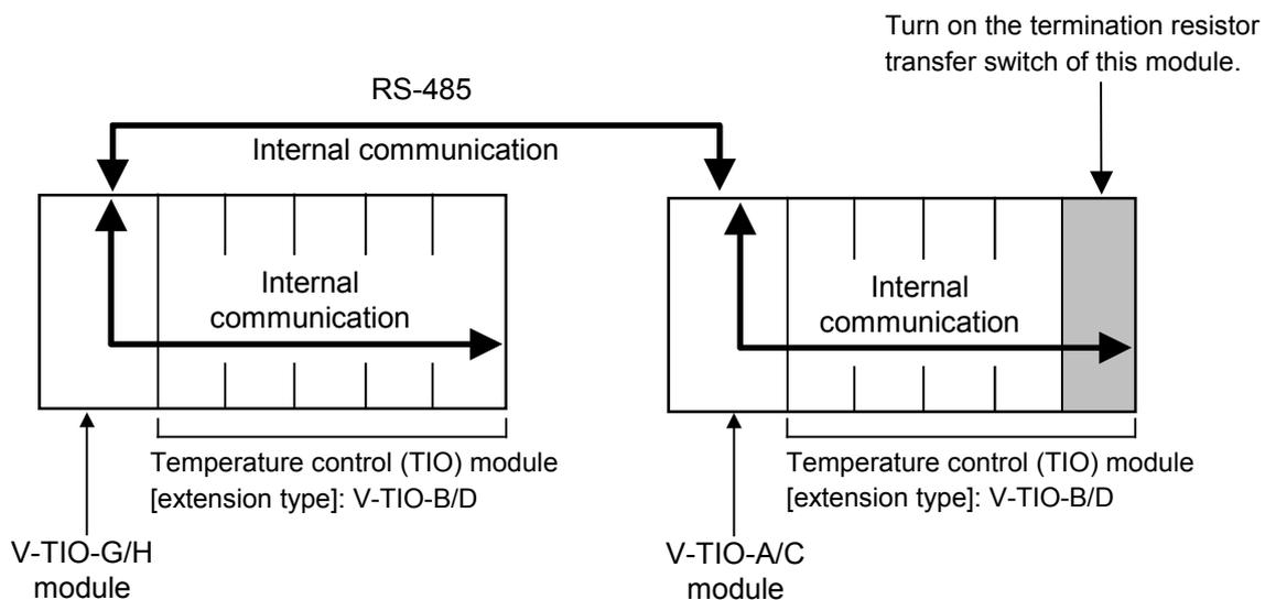
● **Transfer procedure of termination resistor built-in the terminal base**
