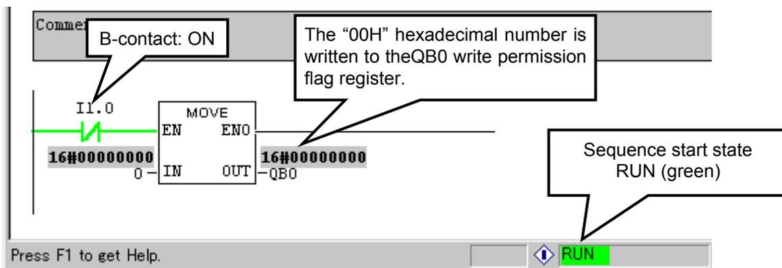
4. Close the contact (DI channel 9) of a digital input module of PLC.
