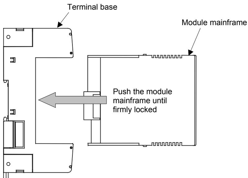
Mounting the module mainframe
