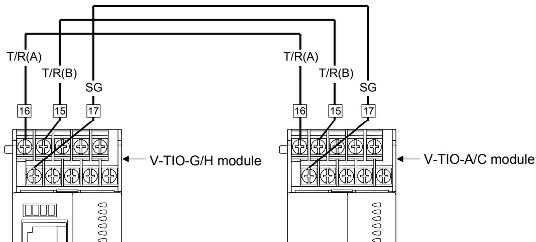
● Communication terminal number and signal details (V-TIO-G/H, V-TIO-A/C)
