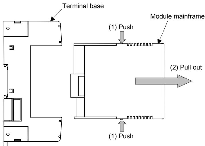
Removing the module mainframe
