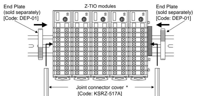
\* It is recommended to use a plastic cover on the connector on both sides of the mounted modules for protection of connectors.
