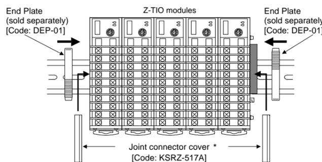
\* It is recommended to use a plastic cover on the connector on both sides of the mounted modules for protection of connectors.
