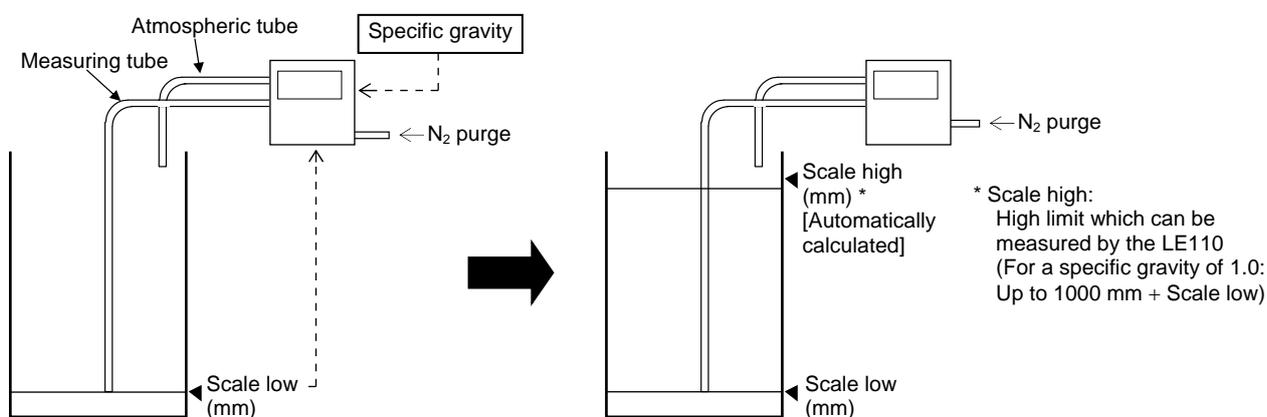
The pressure at each liquid level is measured in accordance with the pressure corresponding to the scale low and the gain called "specific gravity" to calculate the liquid level.
