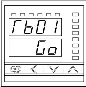
When the setting is finished, the display will automatically go to the next Linearizing table setting.
