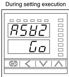
This is the display of the liquid level (actual liquid pressure) captured to activate Output 2.
