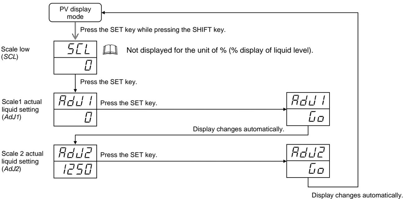
To return to the PV display mode before adjustment is performed, press the SET key while pressing the SHIFT key.
