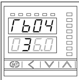
Set the liquid volume corresponding to the liquid level at the fifth point.
