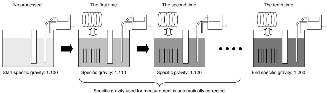
The start specific gravity is set by Specific gravity setting (SG).
