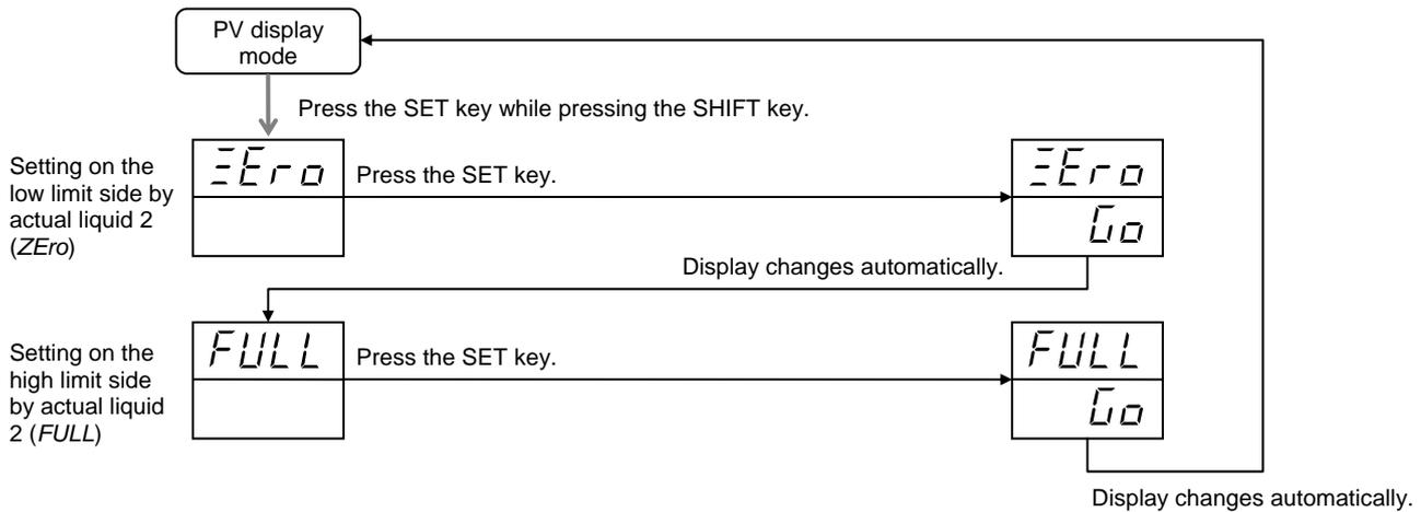
To return to the PV display mode before adjustment is performed, press the SET key while pressing the SHIFT key.
