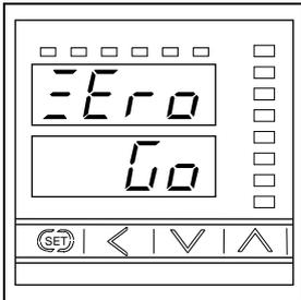
This is the display of the pressure captured at which 0 % is displayed.
