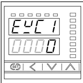
The transistor status (on or off) is selected in the Output 1 activating state (when the output lamp lights).
