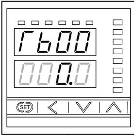
Set the liquid volume corresponding to the liquid level at the first point (minimum value).
