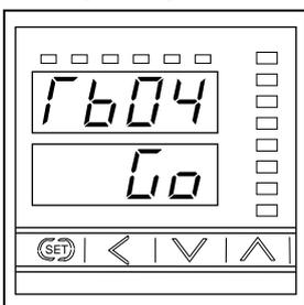
When the setting is finished, the display will automatically return to PV display mode.
