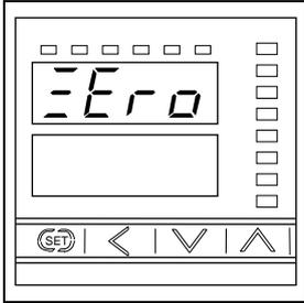
This is the parameter used for capturing the pressure at which 0 % is displayed.
