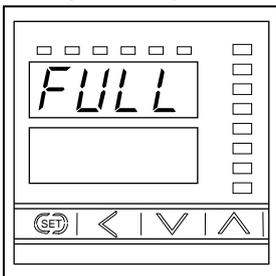
This is the parameter used for capturing the pressure at which 100 % is displayed.
