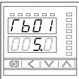
Set the liquid volume corresponding to the liquid level at the second point.
