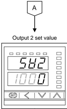
This is the parameter to set the liquid level of activating the output 2.
