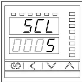
Set the scale low value. Set the distance between the end of the measuring tube and the bottom of the tank used.
