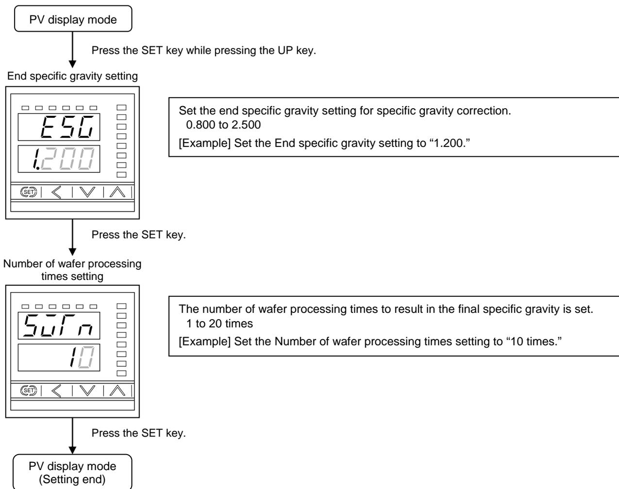
☞ For the Specific gravity correction setting mode, refer to the **6.5.7 Specific gravity correction setting mode (P. 43)**.
