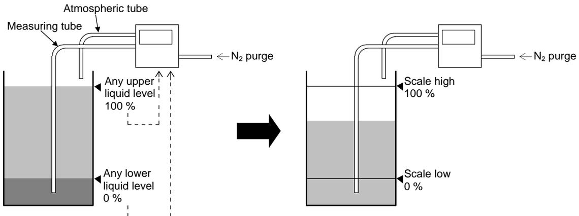
The pressures corresponding to the upper and lower liquid levels are converted to liquid levels of 0 and 100 % and then are displayed.
