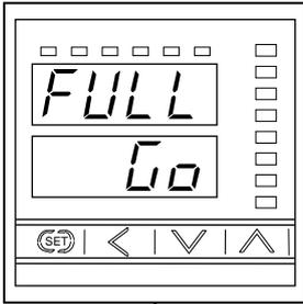
This is the display of the pressure captured at which 100 % is displayed.
