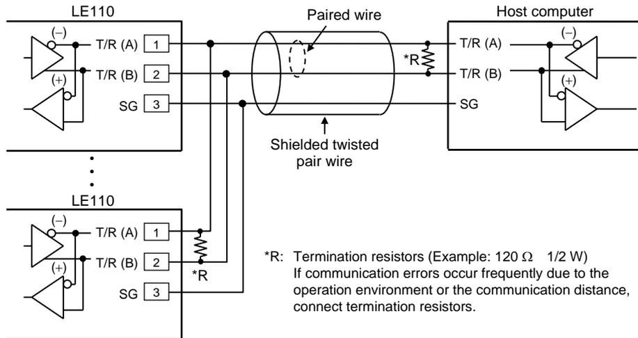
\*R: Termination resistors (Example: 120 Ω 1/2 W)
