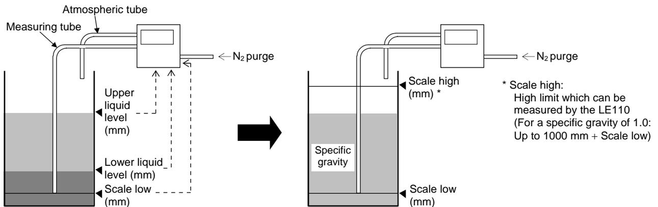
The liquid level is calculated by using the ratio of pressure to height and the height set on each of the upper and lower sides.
