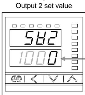
The liquid level captured to activate Output 2 is displayed on the set value display unit.
