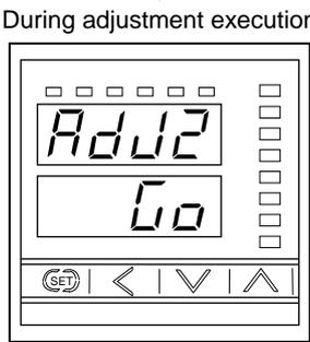
This is the display during adjustment execution of Scale 2 actual liquid setting. The LE110 captures the pressure corresponding to the actual liquid volume at Scale 2 actual liquid level setting of "1000" mm.
