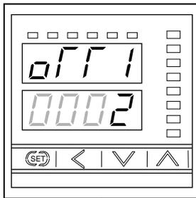
Set the time until output 1 is turned on after measured value enters output area.
