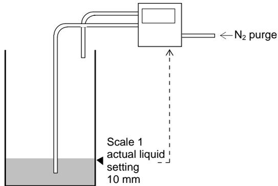
Fill the actual liquid in the tank so that the height of Scale 1 actual liquid setting becomes 10 mm.
