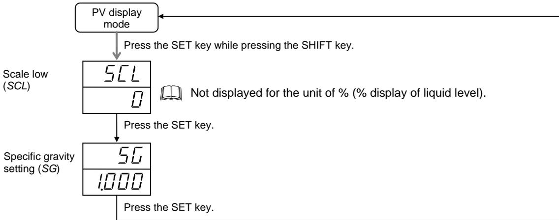
For the operating method of span setting by specific gravity, refer to the **6.4.4 item, ■ Span setting by specific gravity (P. 19)**.
