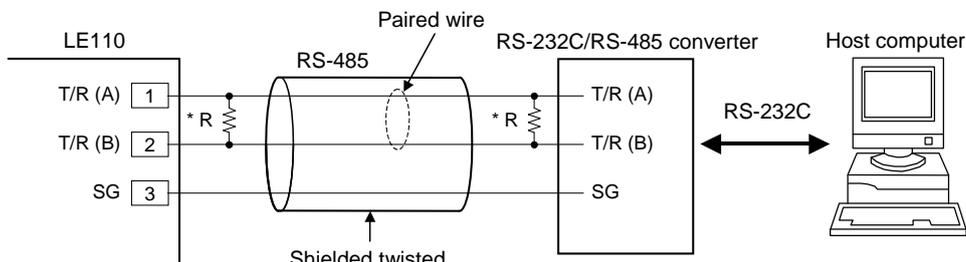
\*R: Termination resistors (Example: 120 Ω, 1/2 W)
