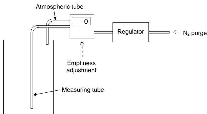
📖 A change in the Number of empty adjustment decision times (Factory set value: 10 times) enables the empty adjustment satisfying the measured object. If the atmosphere at the tube head is unstable (the input value fluctuates) during the empty adjustment, no normal adjustment may be performed to cause an error (Err 16). In such a case if the number of empty adjustment decision times is made smaller, the empty adjustment can be normally performed.
