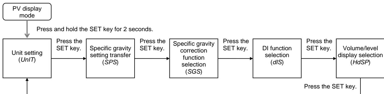
To return to the PV display mode, press and hold the SET key for 2 seconds.
