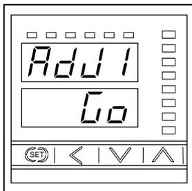
This is the display during adjustment execution of Scale 1 actual liquid setting. The LE110 captures the pressure corresponding to the actual liquid volume at Scale 1 actual liquid level setting of "10" mm.
