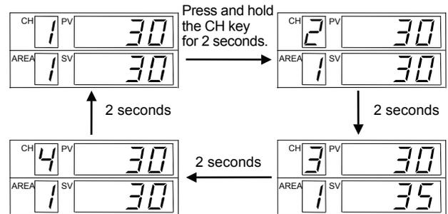
When scanning PV/SV corresponding to channel 1 to channel 4 (channel 3: unused channel) in the control area 1 at 2 seconds intervals:
