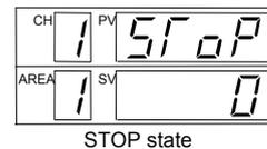
2. The mode is changed to STOP from RUN. The PV display shows the characters of showing the relevant STOP state.
