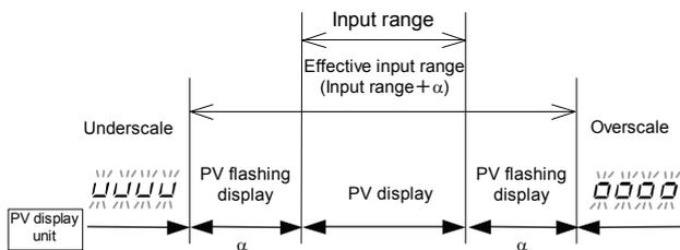
$\alpha$ : The range to be displayed differ depending on the input type or the setting limit.
