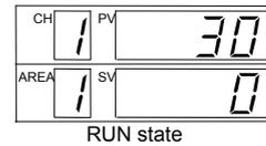
1. Press and hold the <R/S key for 1 second in PV/SV monitor mode.
