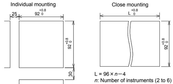
For mounting of the MA900/MA901, panel thickness must be between 1 to 10 mm. When mounting multiple MA900/MA901s close together, the panel strength should be checked to ensure proper support.
