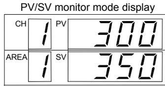
Indicates that PV corresponding to channel 1 within the control area is 300 °C
