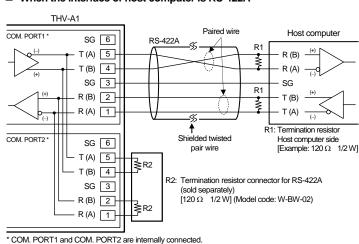
The six-pin type modular connector should be used for the connection to the THV-A1.
