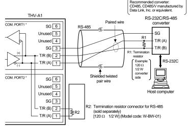
\* COM. PORT1 and COM. PORT2 are internally connected
