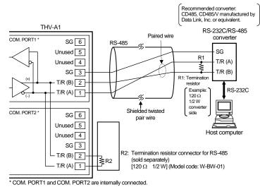
The six-pin type modular connector should be used for the connection to the THV-A1. Recommended manufacture and model: Hirose Electric, TM4P-66P
