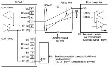
\* COM. PORT1 and COM. PORT2 are internally connected
