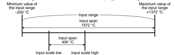
When outside the input scale range, the PV display flashes. The alarm setting range is within the input scale range.
