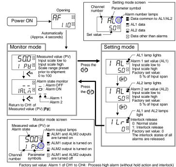
Factory set value: Alarm 1 of CH1 to CH4: Process high alarm (without hold action and interlock)
