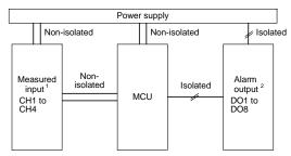
Measured inputs (CH1 to CH4) are not mutually isolated.
