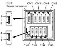
CN2: Sensor input 1 connector CN3: Sensor input 2 connector CN4: Sensor input 3 connector CN5: Sensor input 4 connector
