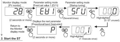
Turn off the power once and turn it on again. The ST will automatically start (During ST execution: AT lamp lights). When the calculation and setting of PID values is completed, setting of the ST screen will automatically change to "0." (ST is completed: AT lamp turns off)
