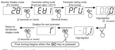
If the set value of Fine tuning is returned to "0: Unused," Fine tuning correction will no longer be applied to control
