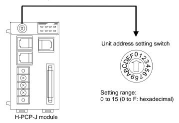
Up to 4 SR Mini HG SYSTEMs can be connected to a PLC communication port. Therefore the data memory address uses the 4 SR Mini HG SYSTEMs as a group. The SR Mini HG SYSTEMs connected to the same PLC communication port sets the address in the same group.
