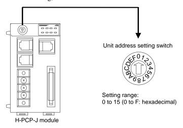
Up to 16 SR Mini HG SYSTEMs can be connected to a PLC communication port.
