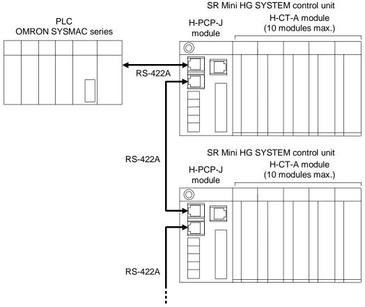
Up to 16 control units per communication port of PLC
