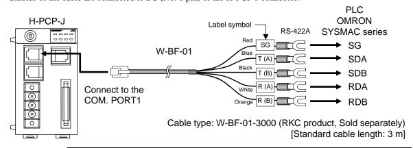
When wiring is to be made with W-BF-01 cable, connect as instructed in the above picture. (Just use the label symbol for leadwire identification and ignore the contents.)
