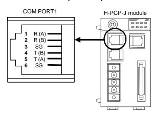
Connector pin number and signal details (RS-422A)
