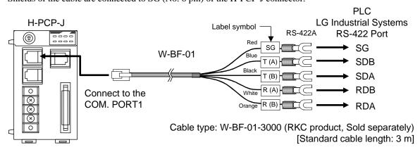
When wiring is to be made with W-BF-01 cable, connect as instructed in the above picture. You do not need to reverse the signal polarity of A and B. (Just use the label symbol for leadwire identification and ignore the contents.)
