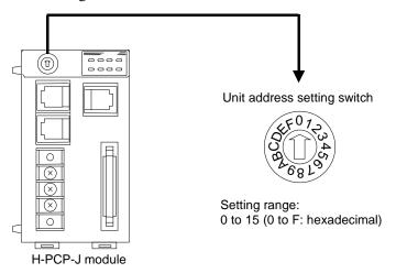
Up to 4 SR Mini HG SYSTEMs can be connected to a PLC communication port. Therefore the file register address uses the 4 SR Mini HG SYSTEMs as a group. The SR Mini HG SYSTEMs connected to the same PLC communication port sets the address in the same group.
