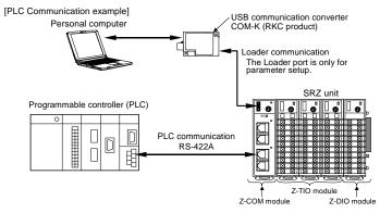
This manual describes the preparation for conducting PLC communication between the Z-COM and PLC For the data map, Host communication, the installation, the detail handling procedures and various function settings, please read if necessary the following separate manuals.
