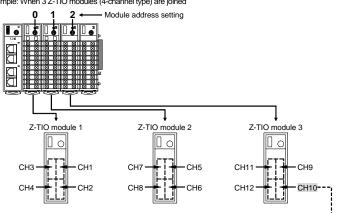
• Z-TIO module 3: The temperature control channel number used for communication of channel 2 <  $2 \times 4 + 2 = 10$
