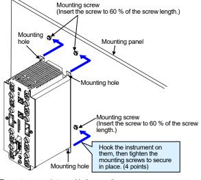
The customer needs to provide the mounting screws M4 size pan-head screws with captive washer and spring washer (Length: 8 mm or longer)...
