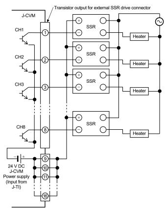
W-CF-S01-AC output cable for transistor (RKC product) can be used as connecting cable (sold separately).
