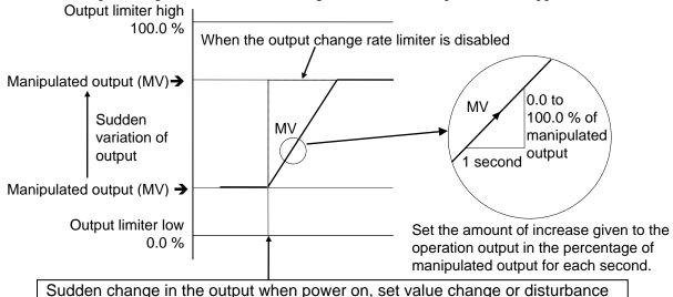
The output changes at specific rates set by output change rate limiter (up) even under the situations where a sudden output change would occur without output change rate limiter function. There is also independent output change rate limiter (down).
