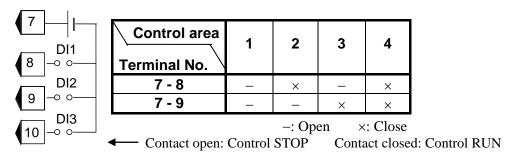
Type 3: Control RUN/STOP selection, Alarm interlock release specifying and Memory area selection
