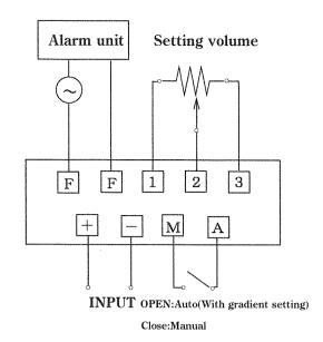
5-3. Auto (With gradient setting) /Manual mode For the type with the optional added, (Cord:-1), it is possible to switch between automatic and manual by using the attached variable resistor and a selector switch. (Selector switch to be supplied by the user.)
