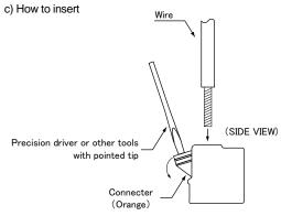
Insert the connector lever as in the illustration and insert the power cord. If the power cord is pushed in coercively without placing the lever, it may become the cause of bad contact or disconnection.
