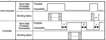
a: Response send time after the controller receives [ENQ] + Interval time
