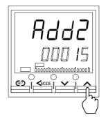
**5.** Press the SET key to store the new set value. The display goes to the next communication parameter. It the SET key is not pressed within one minute, the present display returns to the SV setting & Monitor mode and the value set here returns to that before the setting is changed.
