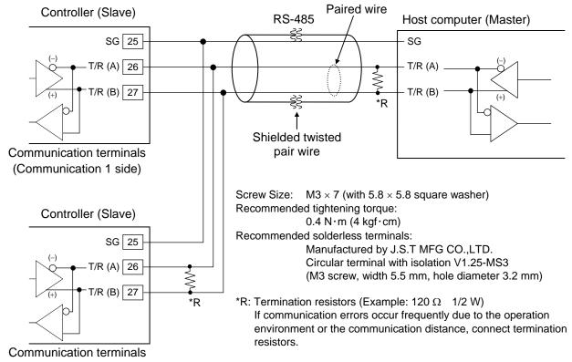
(Communication 1 side) Maximum connections: Up to 31 controllers
