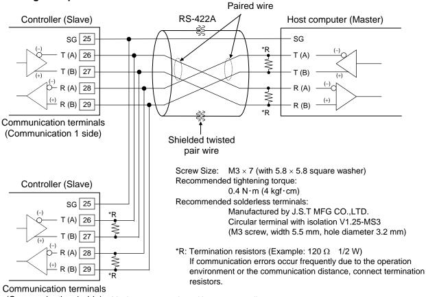
(Communication 1 side) Maximum connections: Up to 31 controllers
