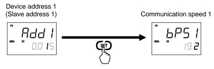
6. Set the Communication speed 1. Press the UP key to select the "38.4." Example: Setting the Communication speed 1 to 38400 bps.
