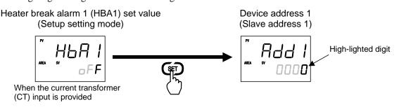
**3.** Set the Device address 1 (slave address 1). Press the UP key to change the number to 5. Example: Setting the Device address 1 (slave address 1) to 15.
