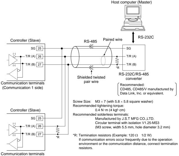
(Communication 1 side) Maximum connections: Up to 31 controllers
