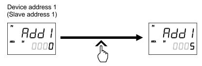
4. Press the shift key to high-light the tens digit, and press the UP key to change the digit to "1."
