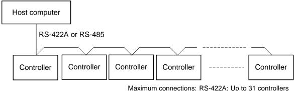
Maximum connections: RS-422A: Up to 31 controllers RS-485: Up to 31 controllers
