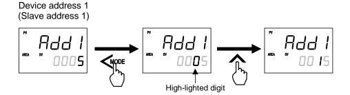
5. Press the SET key to store the new set value. The display goes to the next communication parameter. If the SET key is not pressed within 1 minute, the present display returns to the PV/SV monitor screen and the value set here returns to that before the setting is changed.
