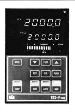
The use of the flat keypad upgrades performance against disturbances like electrostatic noise. It also prevents the dust going into the instrument through the panel.
