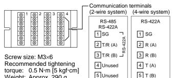
Wiring details of communication cable
