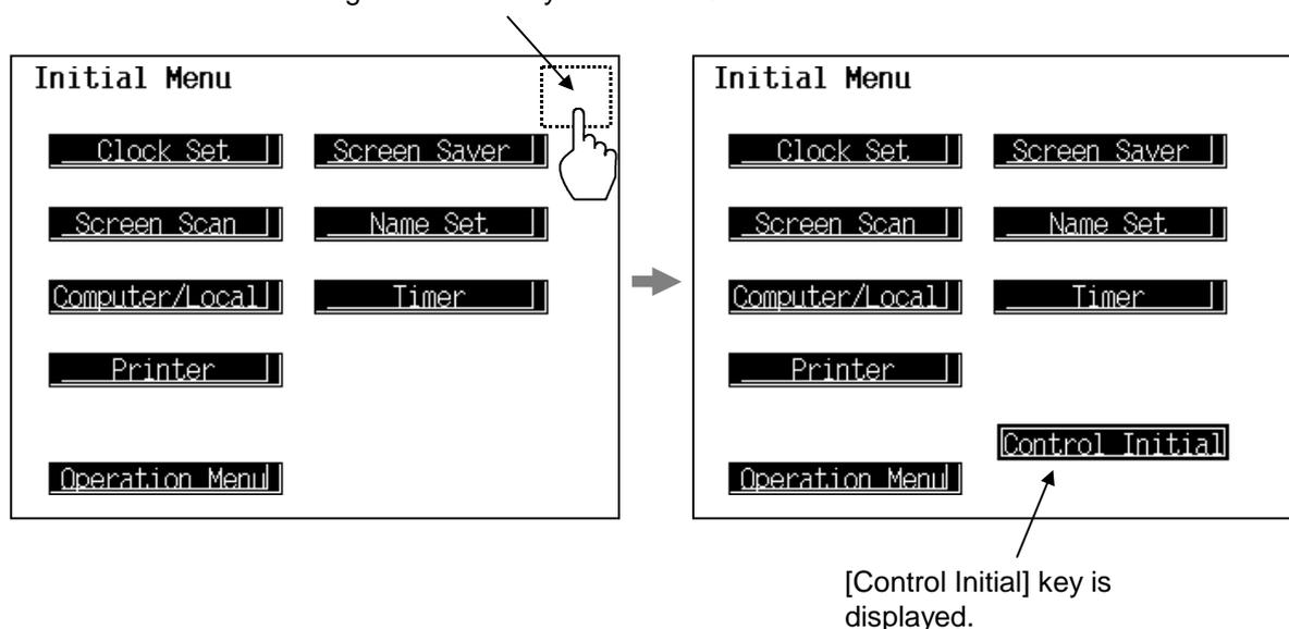
3. Touching the [Controller Initial] key displayed changes the “Controller Initial” screen.
