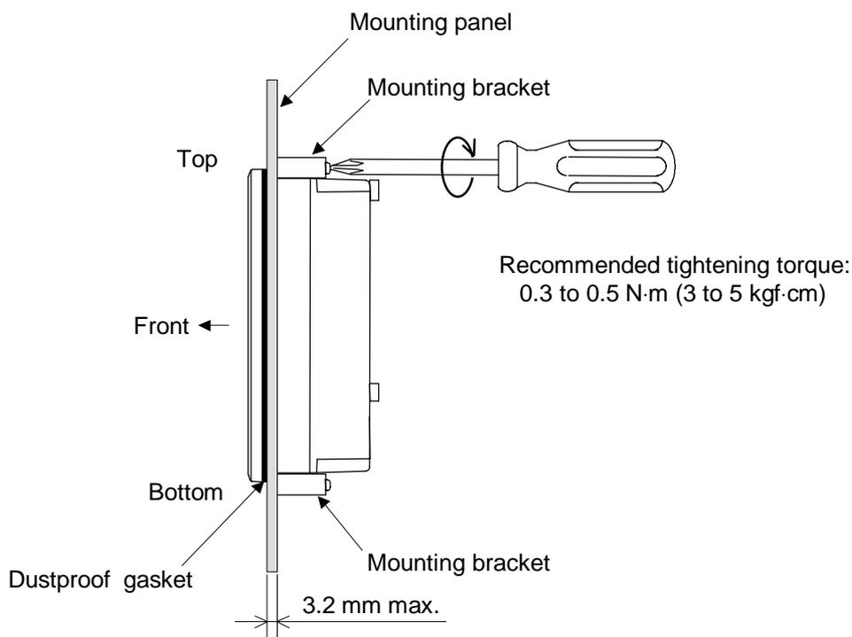
Tightening of the screw (View seen from the side)
