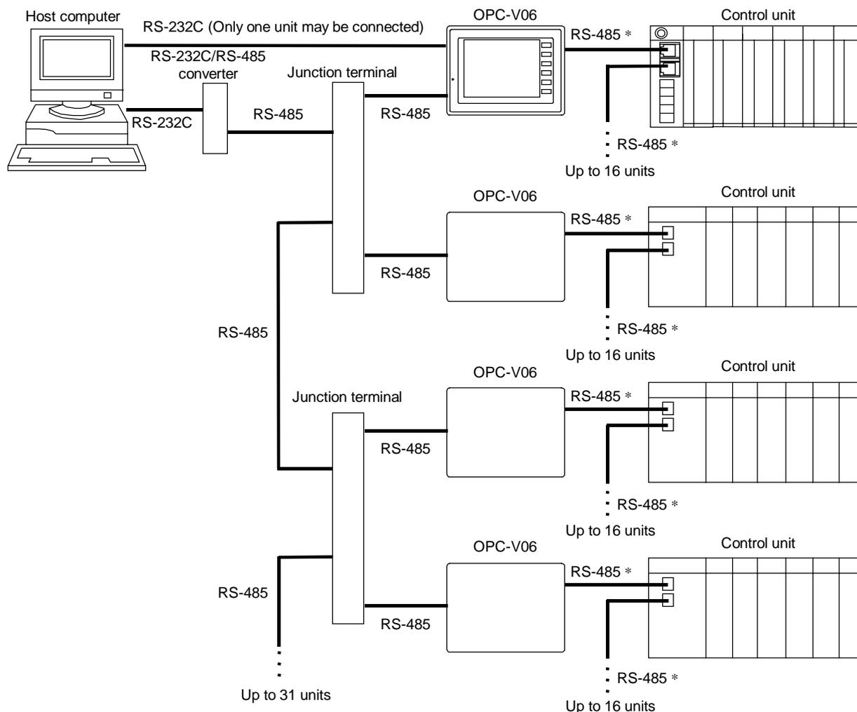
\* The communication interface for SR Mini HG SYSTEM control unit is RS-422A (excluding the RS-485 specification of H-PCP-J). The communication interface is converted RS-422A to RS-485 by connecting modular connector for terminal.
