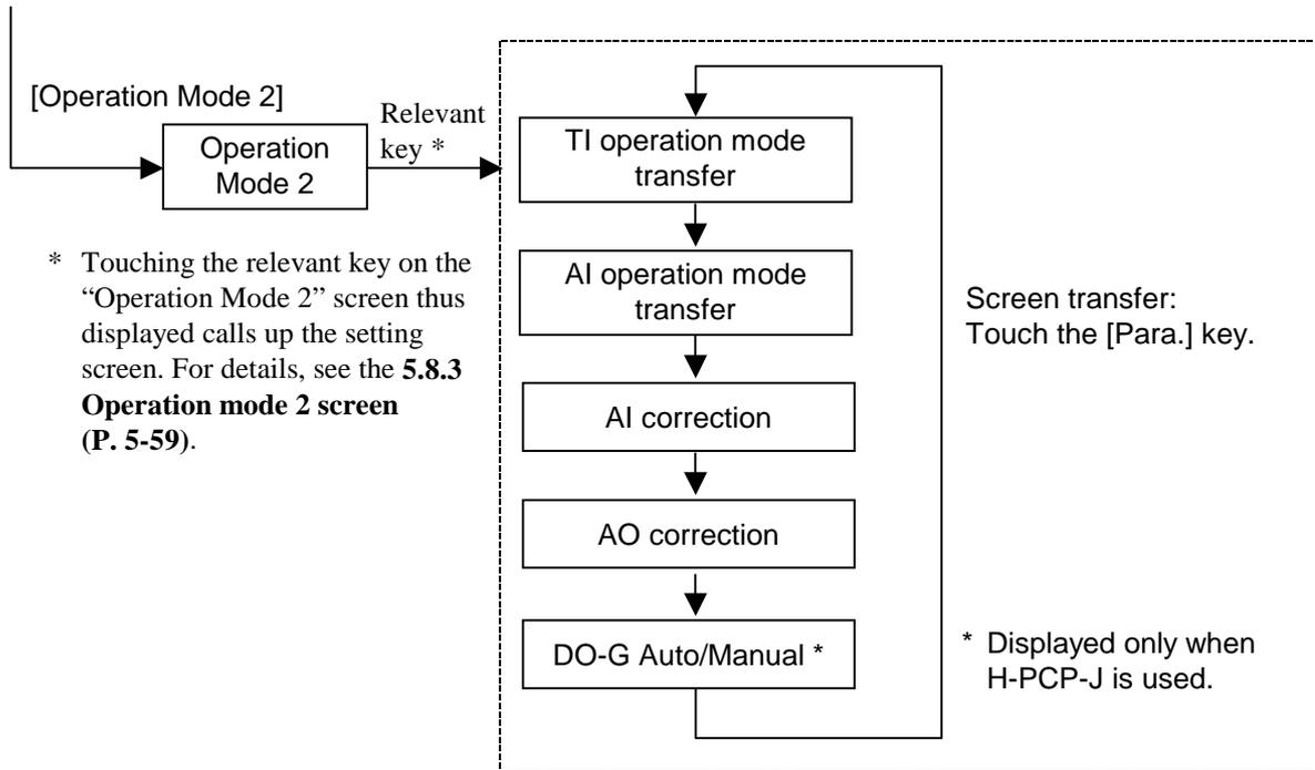
\* Touching the relevant key on the "Operation Mode 2" screen thus displayed calls up the setting screen. For details, see the **5.8.3 Operation mode 2 screen (P. 5-59)**.
