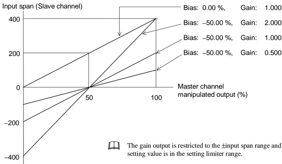
The gain output is restricted to the  $\pm$ input span range and the setting value is in the setting limiter range.
