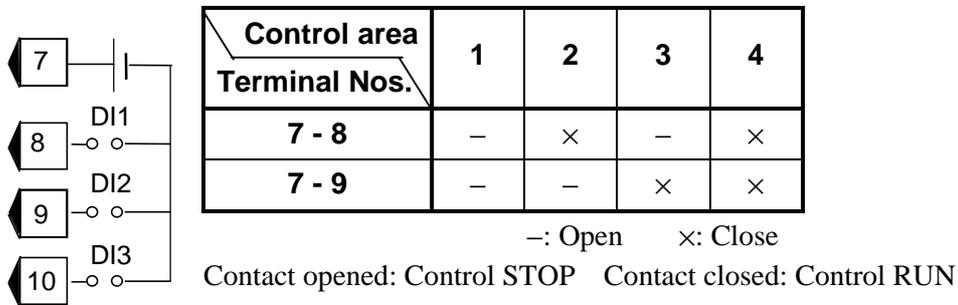
**Control RUN/STOP selection, alarm interlock release specifying and memory area selection (Mode 3):**
