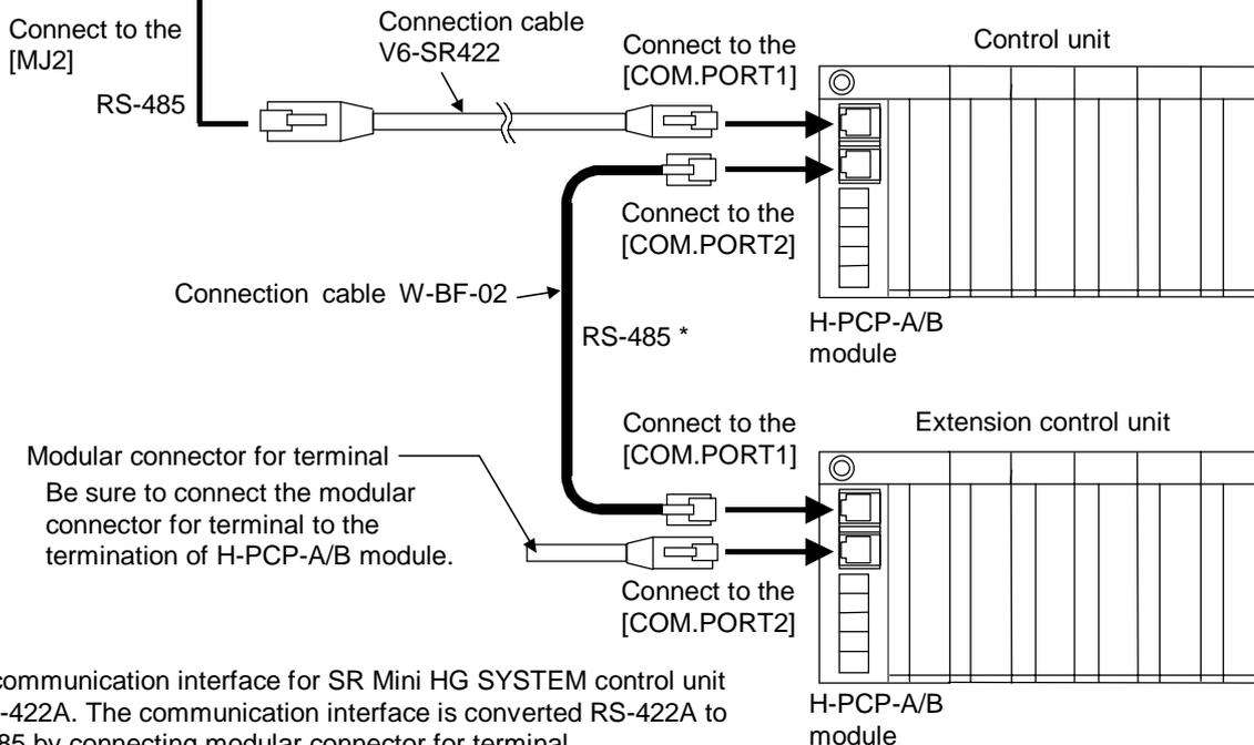
\* The communication interface for SR Mini HG SYSTEM control unit is RS-422A. The communication interface is converted RS-422A to RS-485 by connecting modular connector for terminal.
