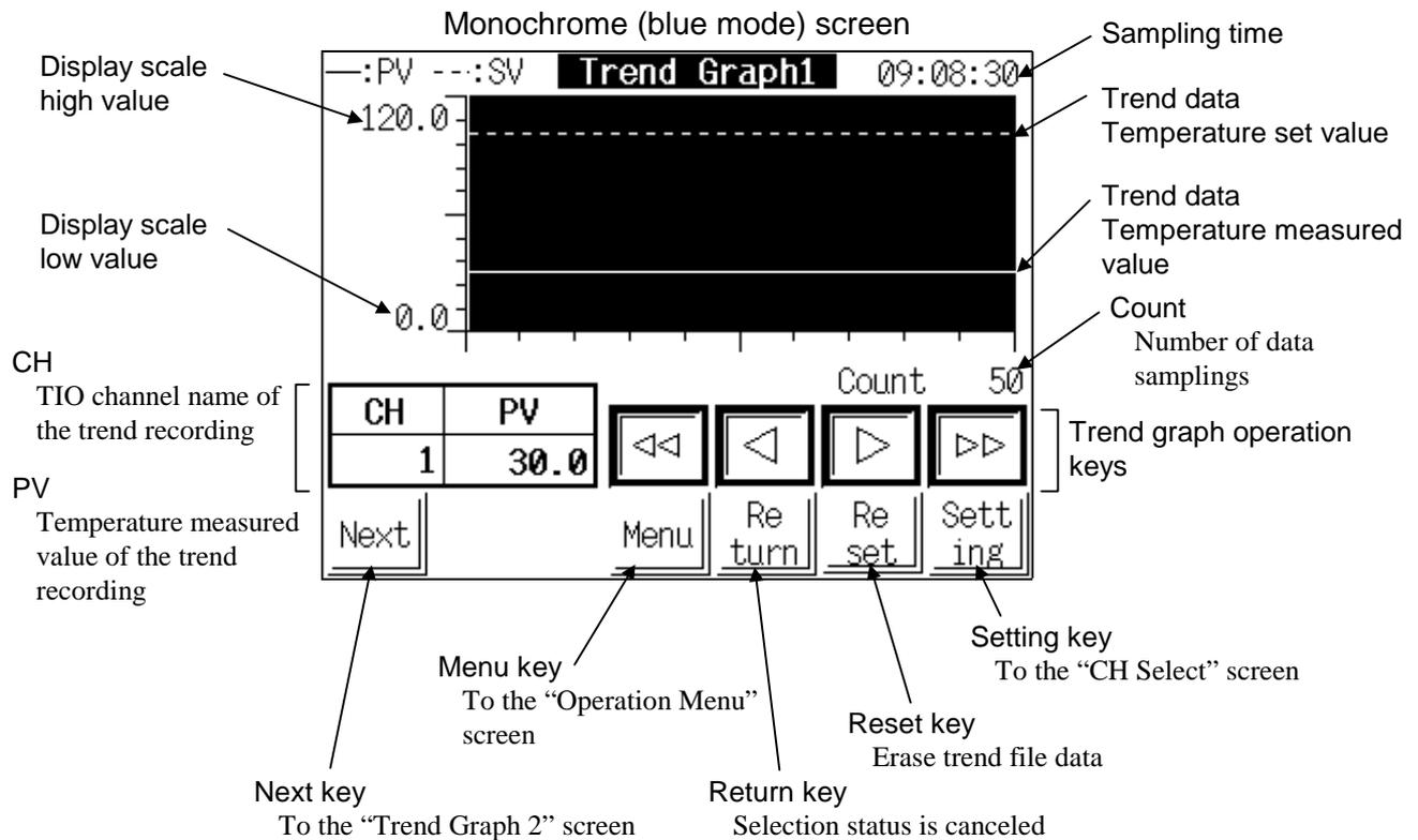
**Sampling time:** Displays the final sampling time or the time that the selected trend data was sampled.
