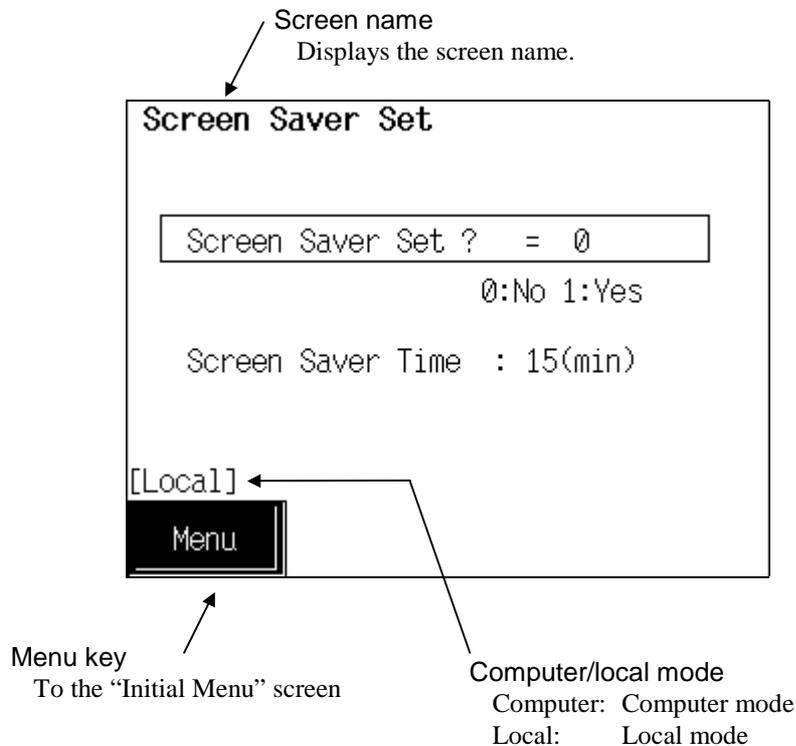
**Screen Saver Set ?:** If key operation is not performed for a specified period of time (15 minutes), it is set whether the function of automatically turning off the display is used or not. If the screen saver has turned off the screen display, touch an any part of the screen to make the display reappear.
