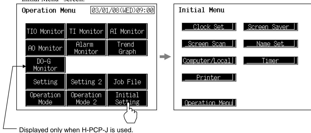
2. Touching the OPC-V initial hidden key more than 8 times in succession displays the [OPC-V Initial] key to make key operation valid.
