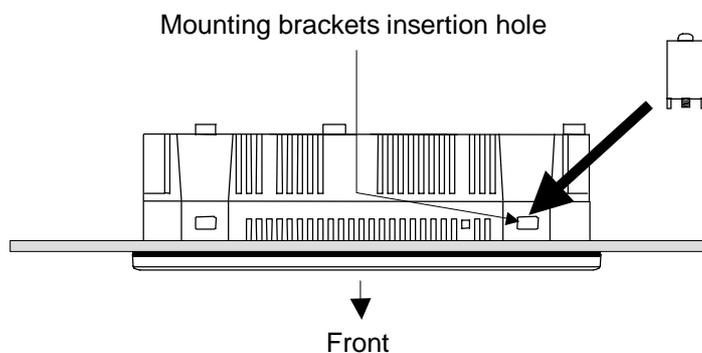
Insertion of mounting brackets (View seen from the top)
