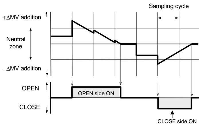
The opening output is not turned on until the control computation result ( $\Delta MV$ ) becomes the neutral zone value or more.
