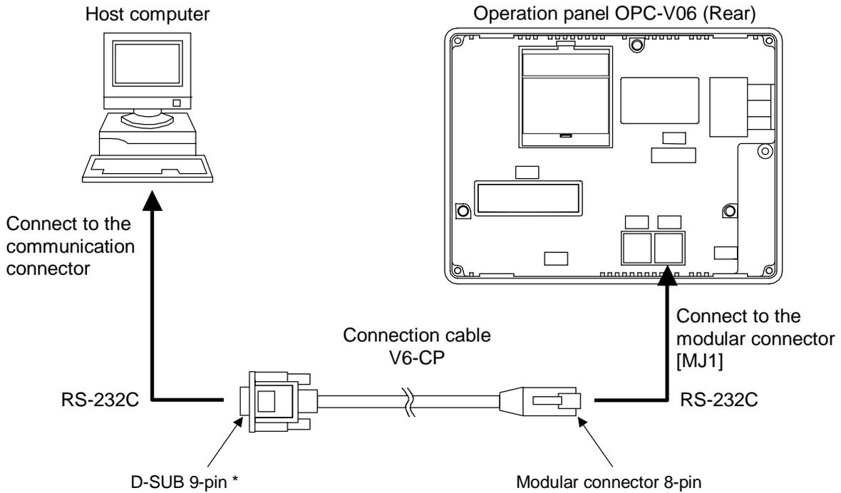
\* Use attached conversion connector (Type: ADP 25-9) when connector of host computer is D-SUB 25-pin.
