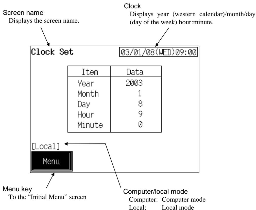
**Setting item:** Set the date and time of the clock function that is built into the operation panel.
