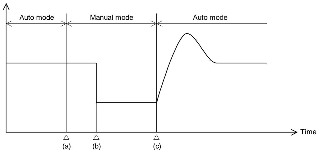
(a) Transfer from auto mode to manual mode. However, when the mode is transferred to manual mode, the manipulated output follows that in auto mode.
