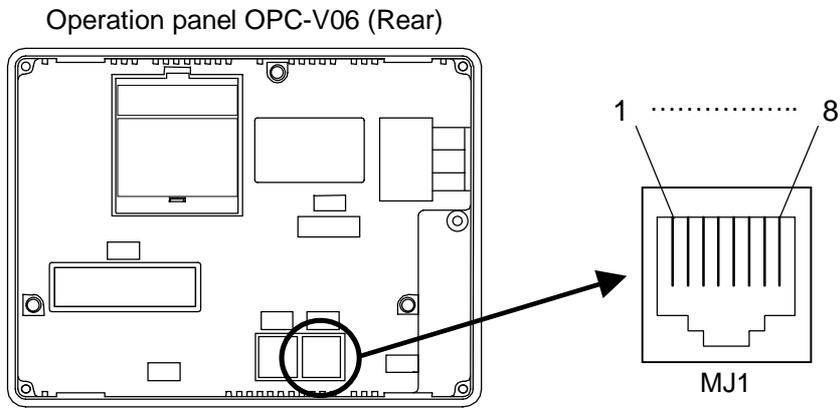
● Connector pin number and signal details [MJ1]
