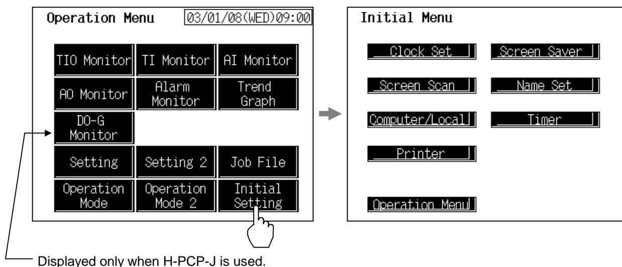
2. Touching the controller initial hidden key more than 8 times in succession displays the [controller Initial] key to make key operation valid.
