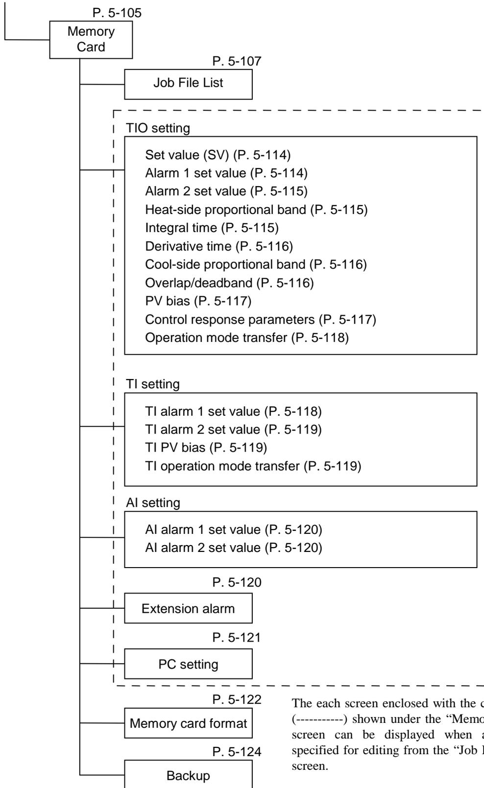
The each screen enclosed with the chain line (-----) shown under the “Memory Card” screen can be displayed when a file is specified for editing from the “Job File List” screen.
