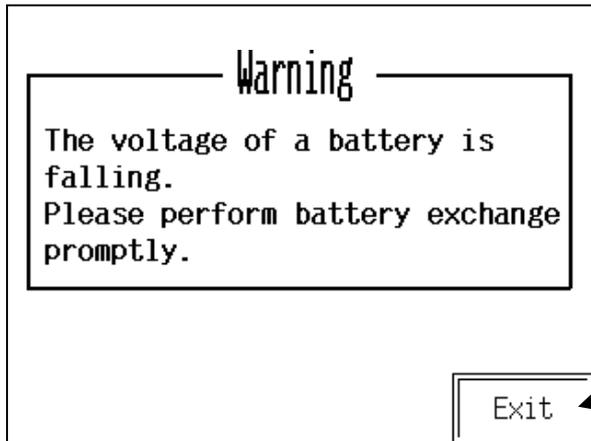
If the battery voltage for SRAM cassette has dropped when the power is turned on, the warning screen will be displayed. Power not supplied SRAM cassette, the data stored in the SRAM cassette may be lost.
