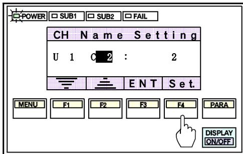
3. After the unit and channel Nos. are set, press the F4 switch(Set.) to display the channel name setting screen. If the above procedure is performed incorrectly, repeat again from Step 1.
