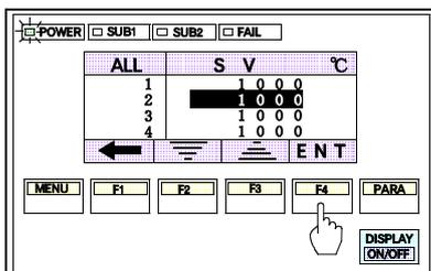
5. Press the F4 switch(ENT) after entering the set value to save it. As a result, the set values of all the channels in the unit selected in Step 1 become the same value.
