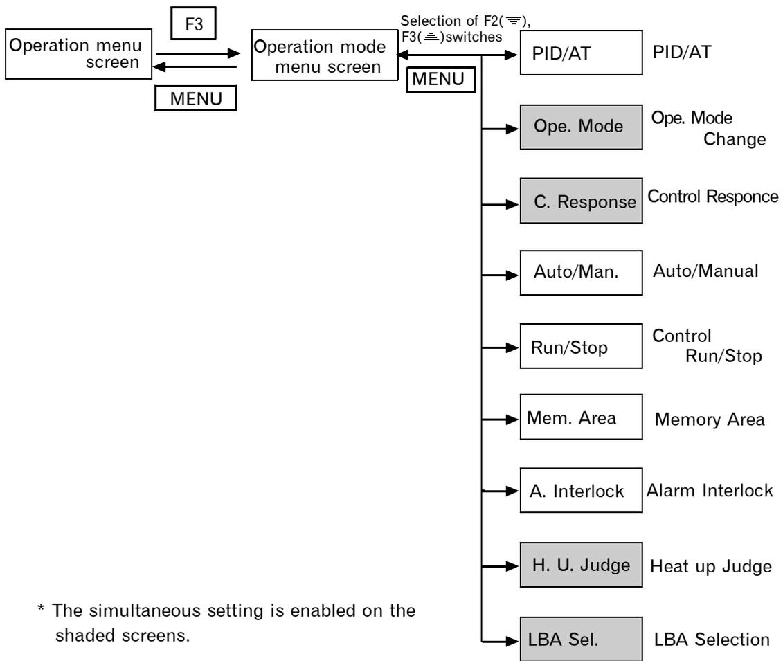
\* The simultaneous setting is enabled on the shaded screens.
