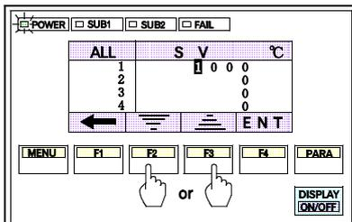
4. Next, move the cursor to the digit to which the desired set value is to be set by pressing the F1 switch(←), then set the set value by pressing the F2(⇒) or F3(⇐) switch. (The example in the figure at the left is when the set value is set to 1000°C.)
