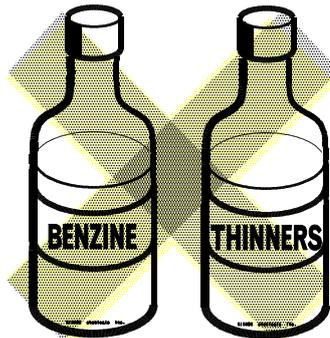
**(Cleaning with a volatile organic solvent will become a cause of switch breakdowns and screen clouding, etc.)**
