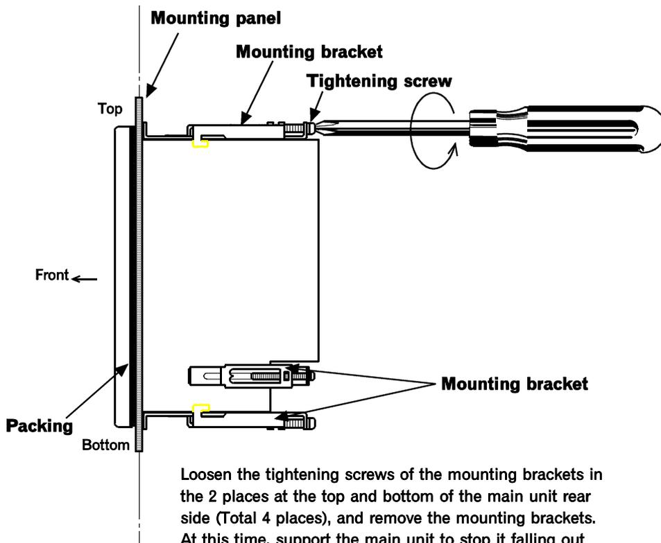
Loosen the tightening screws of the mounting brackets in the 2 places at the top and bottom of the main unit rear side (Total 4 places), and remove the mounting brackets. At this time, support the main unit to stop it falling out from the front face of the mounting panel.
