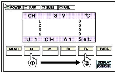
1. Call up the item whose setting need to be changed : select the units to be simultaneously set by pressing the F1 switch (U1) : then press the F4 switch (Set.) .
