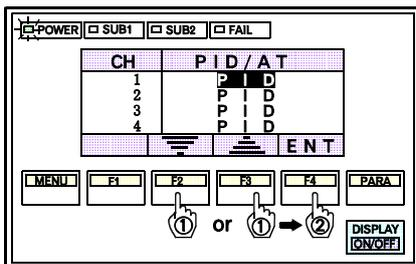
4. Change the data by pressing the F2(≡) or F3(≡) switch, then save it by pressing the F4(ENT) switch. After it is saved, press the MENU switch to return to the setting screen.
