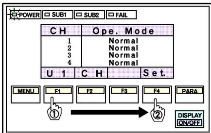
1. Select any unit which is to be simultaneously set by pressing the F1 switch(U1), then press the F4 switch(Set.).
