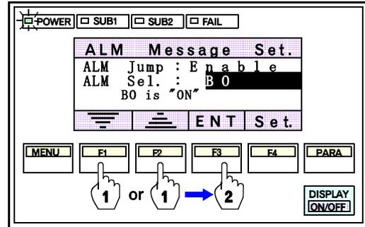
2. Press the F1(≡) or F2 switch(≡) to select the alarm message. Then, press the F3 switch(ENT).
