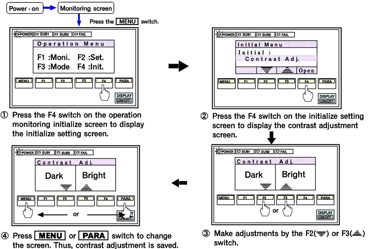
\*The contrast adjustment settings will remain memorized even when the power is turned off.
