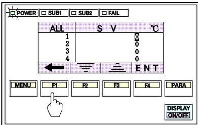
3. In the same way as the normal setting procedure, press the F1 switch(←) once to move the cursor to the 1st digit.
