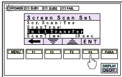
2. Press the F4 switch(ENT) to save the changed set item. After the item is saved, the cursor move to the next set item automatically.
