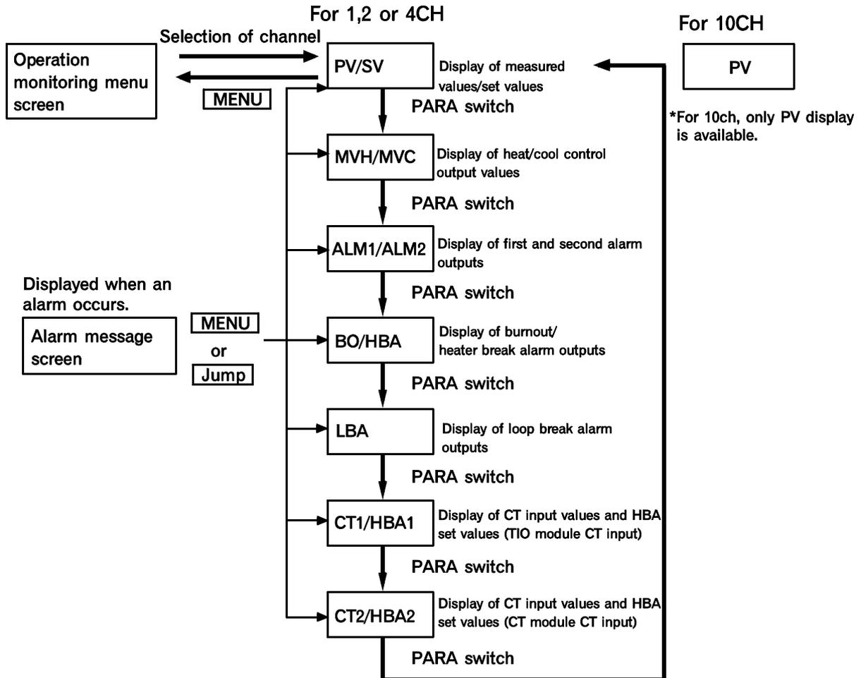
\* If an alarm occurs while 1, 2 or 4CH is being monitored, open the screen to display the current alarm by pressing the hidden switch once.
