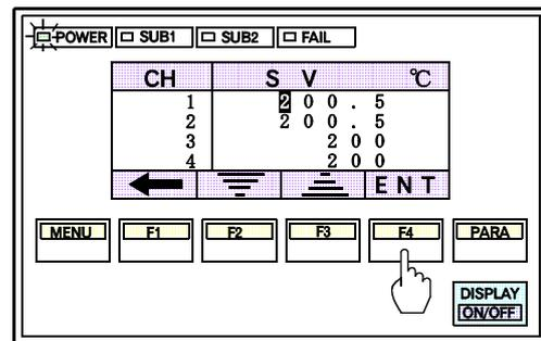
If the set value is saved by pressing the F4 switch(ENT), for the set value without a decimal point, the figures after the decimal point is omitted.
