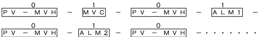
This means that the data on PV (measured value) and heating output which are set to zero is captured first and are updated on the display earlier than the other data. In this manner, use this setting when the monitoring of the small changes on the specific data is necessary. (All values are set to "0" when shipped from factory.)
