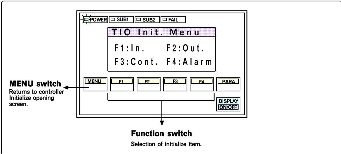
TIO module initialize settings are divided into 4 groups of input, output, control and alarm. Touching the related parameter switch to be initialized changes to the related parameter setting screen.
