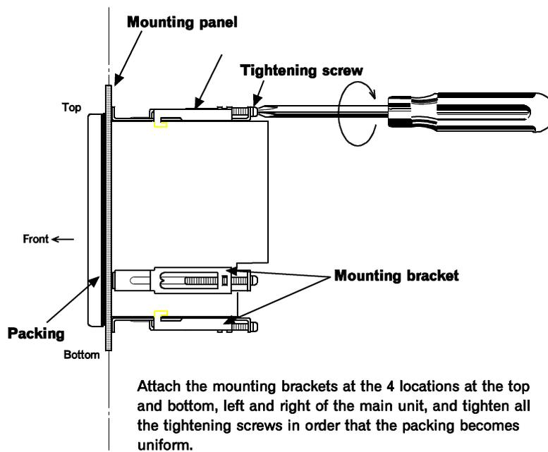
Tightening torque (Recommended value) : 0.3 N·m (3 kgf·cm)
