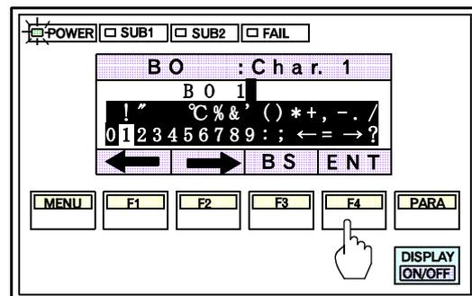
6. After the character is selected, press the F4 switch(ENT) to save the character. If a wrong character is selected by mistake, press the F3 switch(BS) to delete it. Thereafter, select and save the desired character one by one in turn.
