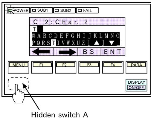
After setting channel 1 as "Tmp01," if channel 2 is to be set as "Tmp02," press the hidden switch A on the channel 2 name setting screen.
