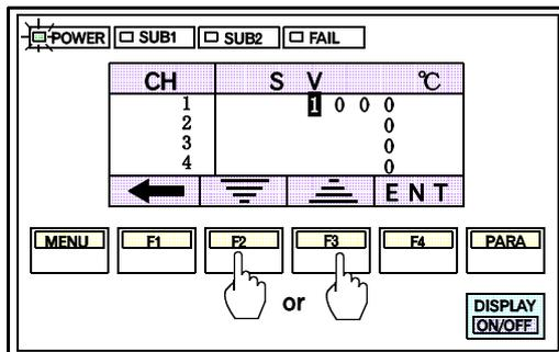
3. Next, move the cursor to digit to which the desired set value is to be set by pressing the F1 switch(←), then set the value by pressing the F2(⇐) or F3(⇒) switch.
