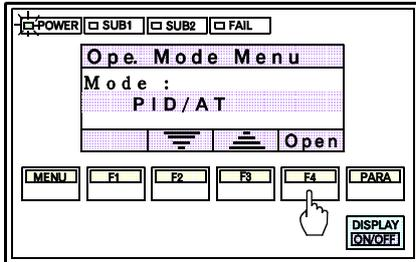
1. Select any time which is to be set, then press the F4 switch (Open).
