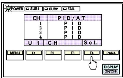
2. Select the desired unit by pressing the F1 switch(U1), also select the desired channel by pressing the F2 switch(CH), then press the F4 switch(Set.) to display the setting change screen.
