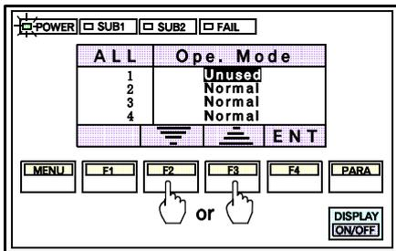
3. Select the mode in which simultaneous setting is to be made by pressing the F2(≡) or F3(≡) switch, then press the F4 switch(ENT). The selected mode is saved. As a result, all the channels of the selected unit are set to the mode thus set.
