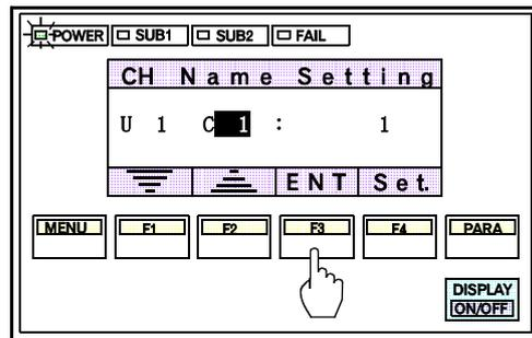
2. Press the F3 switch(ENT) to save the unit No. After the unit No. is saved, the cursor moves to the channel No. Set and save the channel No. in the same way as Step 1.
