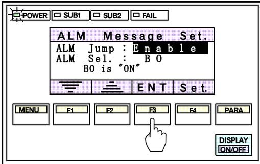
1. Press the F3 switch(ENT) to move the item. The cursor moves to the type of alarm.
