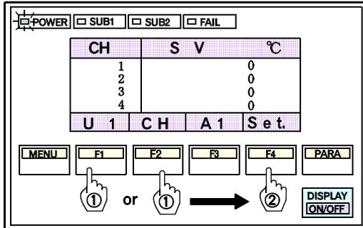
1. Call up any item whose setting is to be changed, select the desired unit by pressing the F1 switch(U1) and the desired channel by pressing the F2 switch(CH), then press the F4 switch(Set.).
