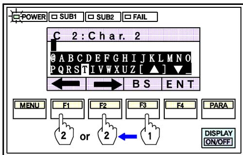
5. Press the F3 switch(BS) to move the cursor, then select the character by pressing the F1 or F2 switch.
