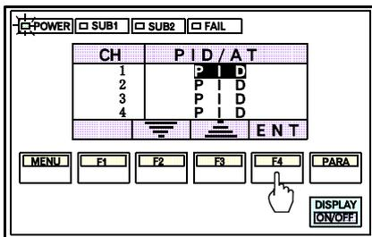
3. Press the F4 switch(ENT) to move the cursor to the channel line to be changed. Every time the F4 switch(ENT) is pressed once, the cursor moves.
