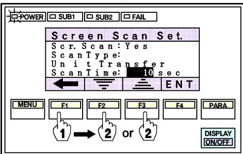
1. Press the F1 switch(←) to move the cursor to the digit to which the desired time to be set. Then, press the F2(⇐) or F3(⇒) switch to set the desired time.
