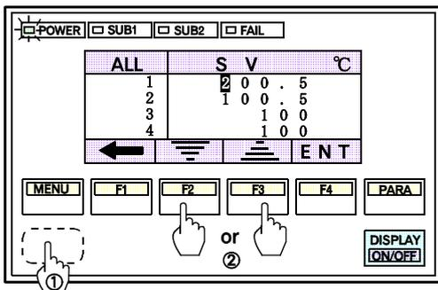
First change CH to ALL by pressing the hidden switch, then set the set value by pressing the F2(⇐) or F3(⇒) switch.
