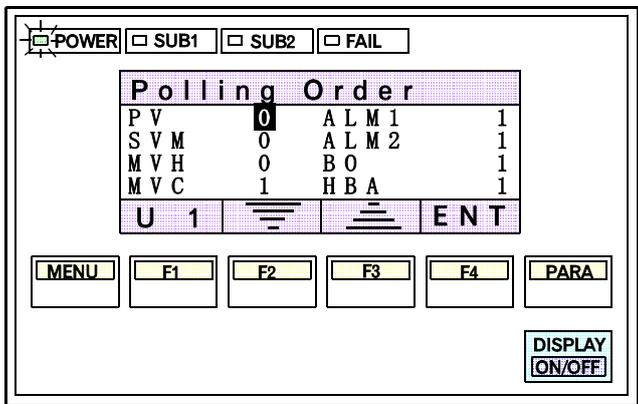
For example if the setting is as shown above, the order of data capture by the operation panel becomes as follows.
