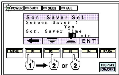
1. Press the F1 switch(←) to move the cursor to the digit to which the desired time is to be set. Then, press the F2(→) or F3(←) switch to set the desired time.
