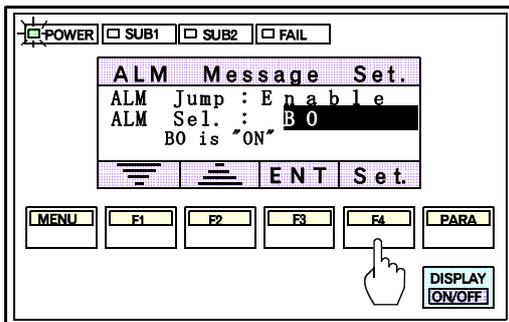
3. After the alarm is selected, press the F4 switch (Set.) to display the alarm message setting screen.
