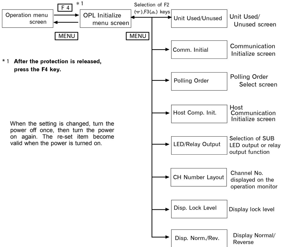
The PARA key cannot be used to move between each item. Therefore, in order to set one of the other items, press the MENU key to return to the OPL initialize menu screen, then select the relevant item.
