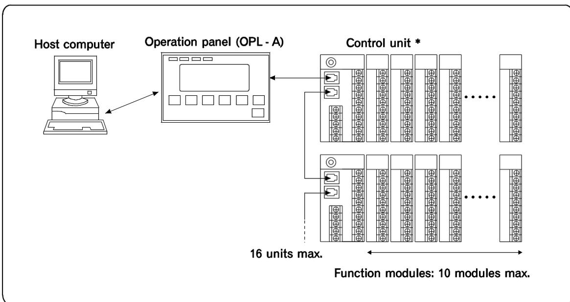
\* Usable modules: M-PCP-A, M-TIO-(A, B, C, D or P type), M-CT-A, M-DI-A, M-DO-A and M-DO-B.
