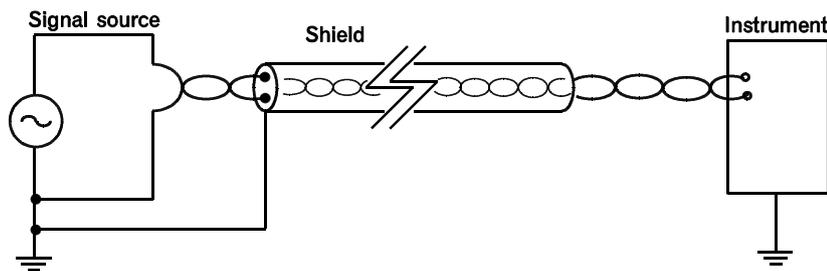
[Example : When signal source is not grounded] Ground the signal source on the instrument side.
