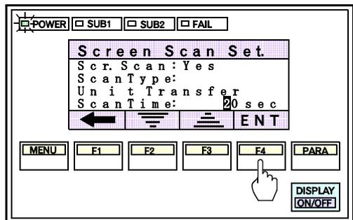
2. Press the F4 switch(ENT) to save the set time. After the time is set, the cursor moves to the first set item automatically.
