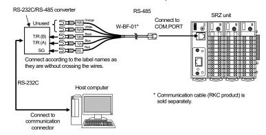
Be sure to insulate the wires that are not used by covering them with insulating tape
