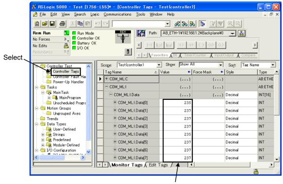
Data of measured value (PV) channels 1 to 8
