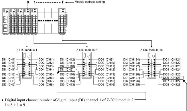
• Digital output channel number of digital output (DO) channel 6 of Z-DIO module 16  $\cdot$  15  $\times$  8 + 6 = 126
