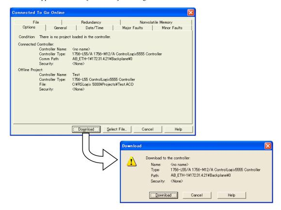
3. "Off line" at the upper left of the test project screen will change to "Rem Run," and I/O communication will be executed. If communication is normal, the display to the right of "Rem Run" will change to Run Mode, Controller OK, Battery OK, and I/O OK.
