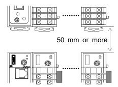
• Depth for modular cables mount type module
