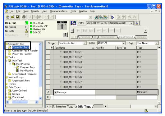
3. Create the program in the screen that appears when "Tasks" → "Main Task" → "Main Program" → "Main Routine" is selected in the tree on the left side of the test project screen.
