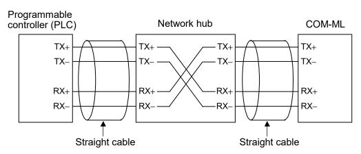
Cross cables may be used depending on the connecting device used. Therefore, follow the instructions for the respective device.
