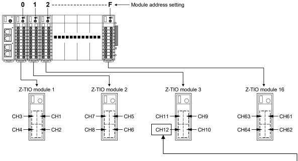
• Z-TIO module 3: The temperature control channel number used for communication of channel 4 - 2 × 4 + 4 = 12
