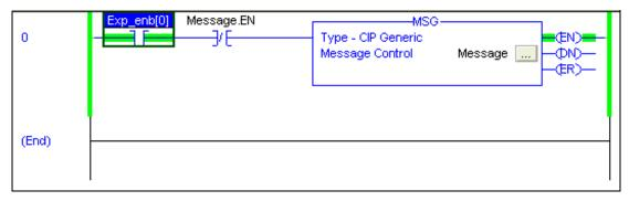
1. Register the "Exp\_enb" relay (contact a), which is the trigger for explicit message transmission, ahead of time in "Tasks" → "Main Task" → "Main Program" → "Program Tags" in the tree at the left side of the test project screen.
