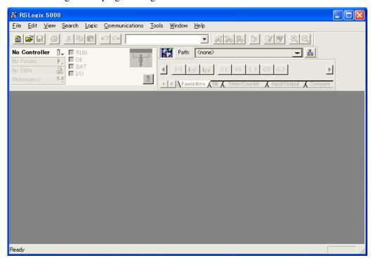
2. Select "New" from the "File" in the menu bar to open the "New Controller" window and create a new project. Configure the following settings in "New Controller."
