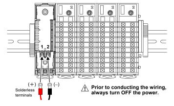
3. Return the module mainframe to the base. This completes the wiring work.
