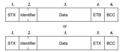
If the length of send data (from STX to BCC) exceeds 128 bytes, it is divided into blocks by ETB. In this case, the succeeding divided data is sent after STX.
