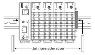
• Be sure the COM-ML and SRZ function modules (Z-TIO and Z-DIO modules) are joined when using them.
