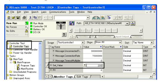
3. Set the value of "Exp\_enb [0]" to "1" in "Tasks" → "Main Task" → "Main Program" → "Program Tags" in the tree at the left side of the test project screen. Explicit message communication will be executed, and the value of set value (SV) channel 2 will be "200."
