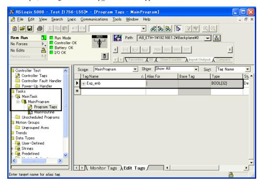
2. Store "Message" in Edit Tags of "Controller Test" → "Controller Tags" in the tree at the left side of the test project screen.
