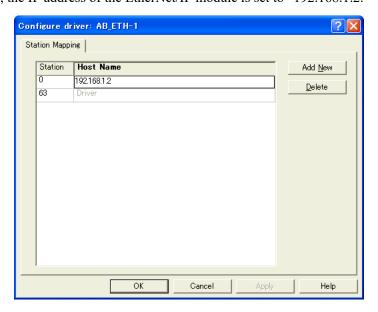
**6.** The "AB\_ETH-1" driver of the EtherNet/IP module is added to "Configured Driver:" of the "Configure Drivers" window.
