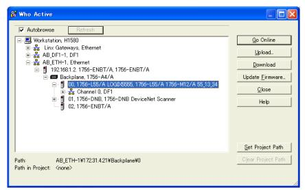
6. Click the [Close] button to store the path that is selected in "Path" on the test project screen.
