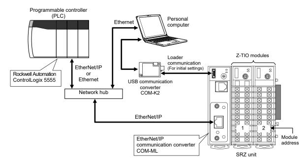
Loader communication is used for the initial communication data settings.
