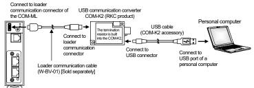
The Loader port is only for parameter setup. Not used for data logging during
