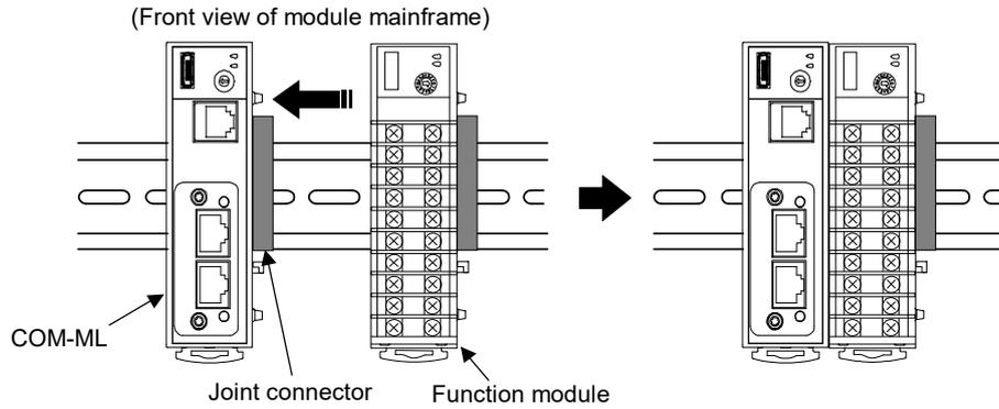
2. Push in the mounting brackets to lock the modules together and fix to the DIN rail.
