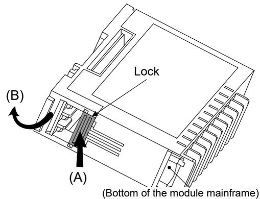
3. Join bases. Then, lock them by pushing in the mounting brackets. (Refer to P. 10)
