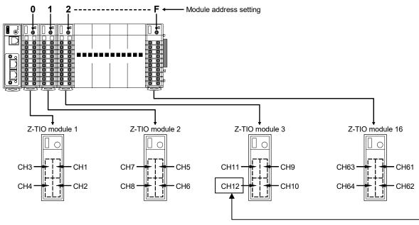
• Z-TIO module 3: The temperature control channel number used for communication of channel 4 --- 2  $\times$  4 + 4 = 12
