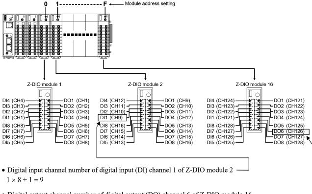
• Digital output channel number of digital output (DO) channel 6 of Z-DIO module 16
