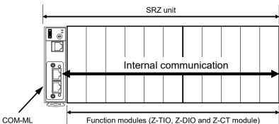
Setting the Z-TIO module address determines the temperature control channel number used for communication.
