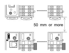
• Depth for modular cables mount type module Space for modular cables must be considered when installing.
