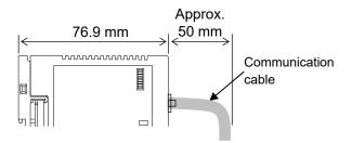
• It is recommended to use a plastic cover on the connector on both sides of the mounted modules for protection of connectors.
