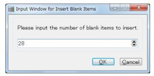
**6.** Blank registers for 28 items are allocated between the monitor group and setting group. The register addresses of the setting group automatically shift by an amount equal to the inserted registers.
