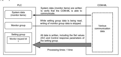
3. When writing is finished, the Monitor request bit will change to "0" to indicate that writing of data to the PLC is finished.
