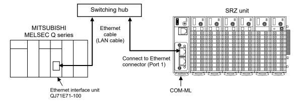
The details of the connectable connector for the PLC, refer to the instruction manual for the used PLC.
