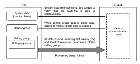
3. When reading is finished, the Setting request bit will change to "0" to indicate that reading of data from the PLC is finished.
