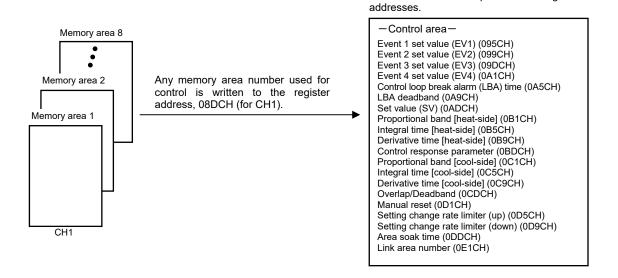
Data corresponding to a specified Memory area number is called up to the CH1 register
