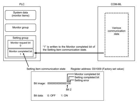
5. If the Monitor request bit is 0 at the timing of the next update of the "Setting item communication state", the Monitor completion bit returns to 0.
