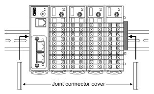
• Be sure the COM-ML and SRZ function modules (Z-TIO, Z-DIO and Z-CT modules) are joined when using them.
