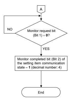
If the Monitor request bit (Bit 1) of the Request command of the PLC register is "**0**," this indicates that writing of data to the PLC is finished.
