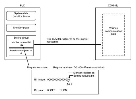
4. When writing is finished, the COM-ML writes the communication state of the setting group to the Monitor completed bit of setting item communication state.
