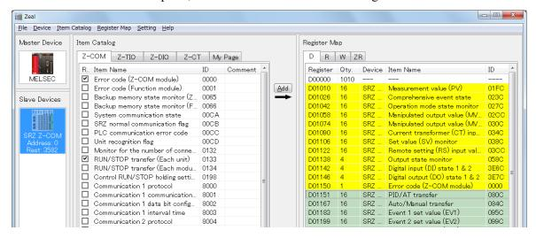
**3.** Click a Z-CT tab of Item Catalog, and display data of the Z-CT module. Register the following data here.
