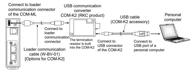
During the loader communication, the COM-ML requires an external power source. The COM-ML will not function on the USB power from a personal computer alone.
