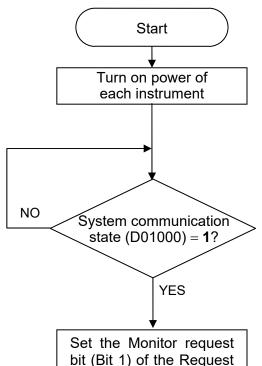
Turn on the power of the SRZ unit, the PLC, and the host computer. The COM-ML starts collecting data on function modules (Z-TIO, Z-DIO and Z-CT modules) jointed from the time when the power is turned on.
