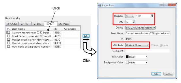
8. Set Heater break alarm (HBA) state monitor and Automatic setting state monitor similarly. Set the register addresses so that they follow in succession after Current transformer (CT) input value monitor.
