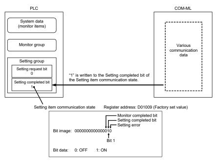
At the timing when the Setting completion bit gets 1 (edge), monitor the setting error flag at the same time.
