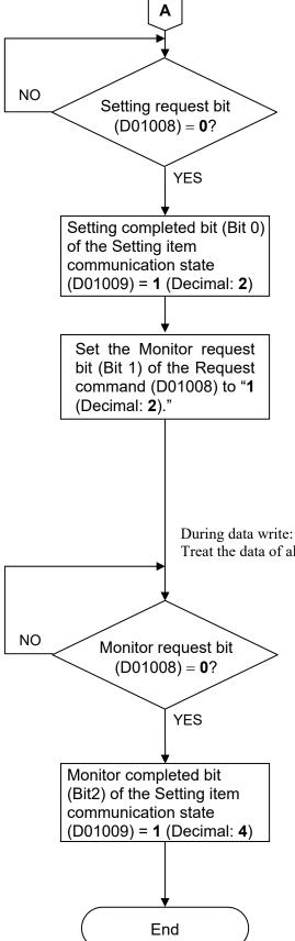
If the Setting request bit (Bit 0) of the Request command (**D01008**) of the PLC register is "**0**," this indicates that reading of data from the PLC is finished.
