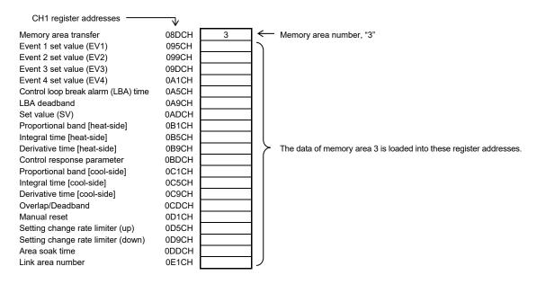
2. Control of CH1 is performed by using data in the register addresses.
