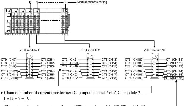
• Channel number of current transformer (CT) input channel 6 of Z-CT module 16 -
