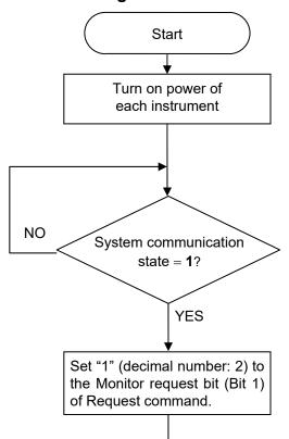
When the power of the SRZ unit is turned on, data collection of the function modules (Z-TIO, Z-DIO and Z-CT modules) joined to the COM-ML starts.
