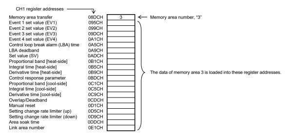
2. Control of CH1 is performed by using data in the register addresses.
