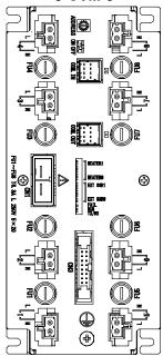
The J-CVM is an SSR output unit designed for heater control system. In addition, an "Output for external SSR drive" is provided for driving the external SSR.
