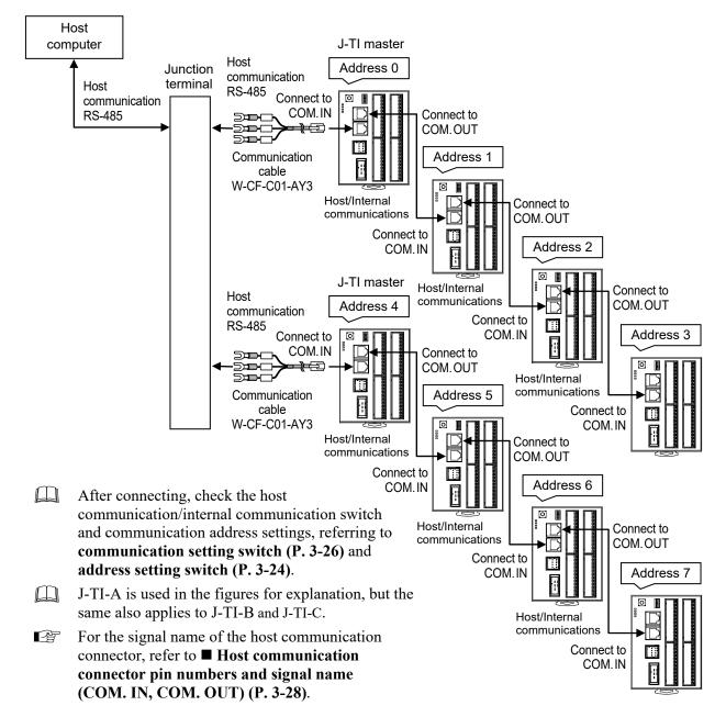
W-CF-C01-AY3 communication cable (RKC product) can be used as communication cable for connecting J-TI to the host computer (sold separately). If noise is a factor, customer should use a twisted pair cable (not included) or something to that effect.
