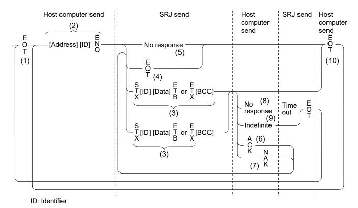
\* When the transmission data (from STX to BCC) of the same identifier is divided by ETB into blocks, the transmission of the remaining data resumes from the divided data following the STX.
