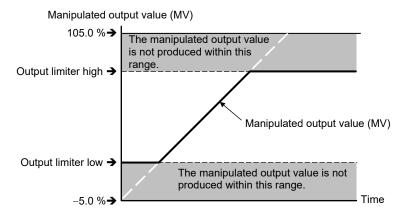
Output limiter is also effective in ON/OFF control.
