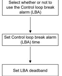
Select whether or not to use the Control loop break alarm (LBA) under Control loop break alarm (LBA) usage selection.
