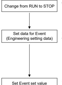
Change the setting to "0: STOP (Control stop)" by RUN/STOP transfer.
