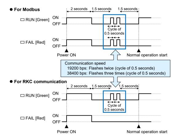
The RUN [Green] lamp and FAIL [Red] lamp are present on the J-TI front panel.
