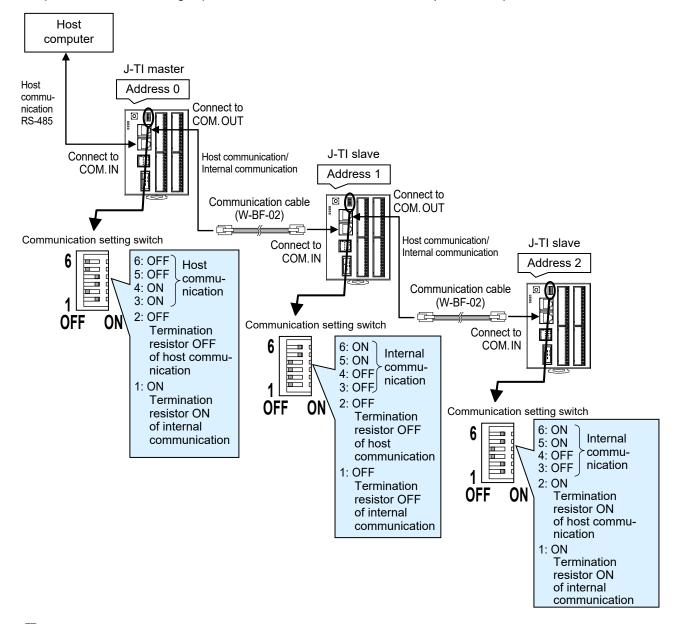
W-BF-02\* communication cable (RKC product) can be used as communication cable for connecting J-TI to J-TI (sold separately). If noise is a factor, customer should use a twisted pair cable (not included) or something to that effect.
