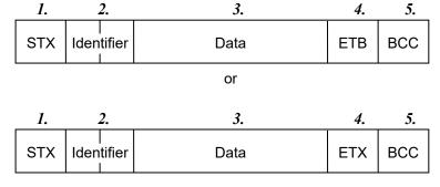
When the transmission data (from STX to BCC) of the same identifier is divided by ETB into blocks, the transmission of the remaining data resumes from the divided data following the STX.
