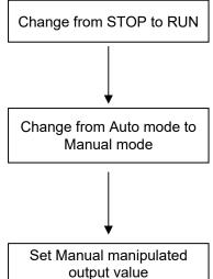
Change the setting to "1: RUN (Control start)" by RUN/STOP transfer.
