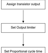
If you use a transistor output for external SSR driving, the temperature input channels are assigned by transistor output selection.
