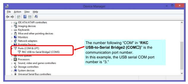
If a yellow question mark appears over the icon of COM-K2 "RKC USB-to-Serial Bridge2 (COM□)," the COM-K2 might not be working normally. Reinstall the COM-K2 USB driver to solve the problem.
