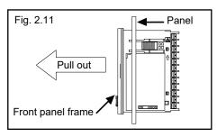
Use long-nose pliers to remove mounting brackets from the instrument that is installed in a narrow place or installed tightly in a vertical position.
