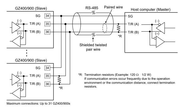
The communication cable and termination resistor(s) must be provided by the customer.
