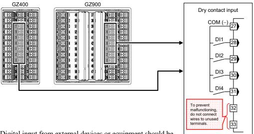
• Digital input from external devices or equipment should be dry contact input. If it is not dry contact input, the input should meet the specifications below.
