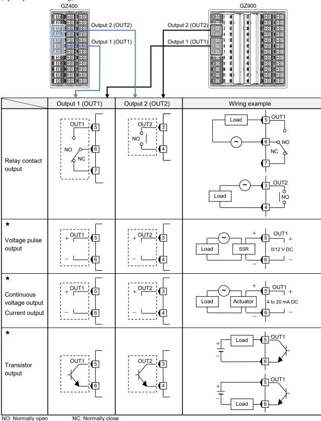
★: To prevent malfunctioning, do not connect wires to unused terminals (terminal No. 7).
