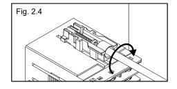
Do not overtighten the screw. It may turn idle. In case the screw has been overtightened to turn idle, loosen the screw, then tighten the screw again until the instrument is firmly fixed.
