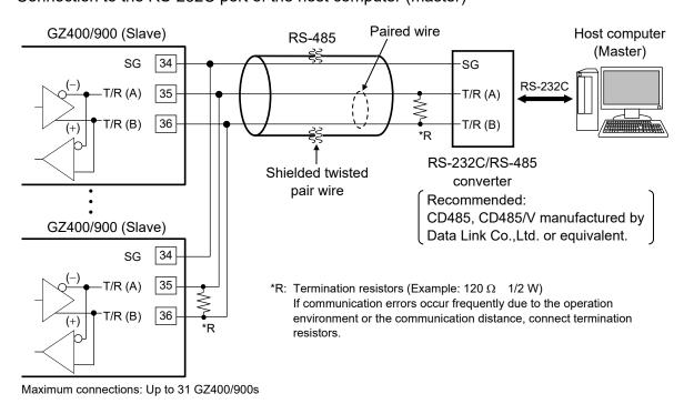
The communication cable and termination resistor(s) must be provided by the customer.
