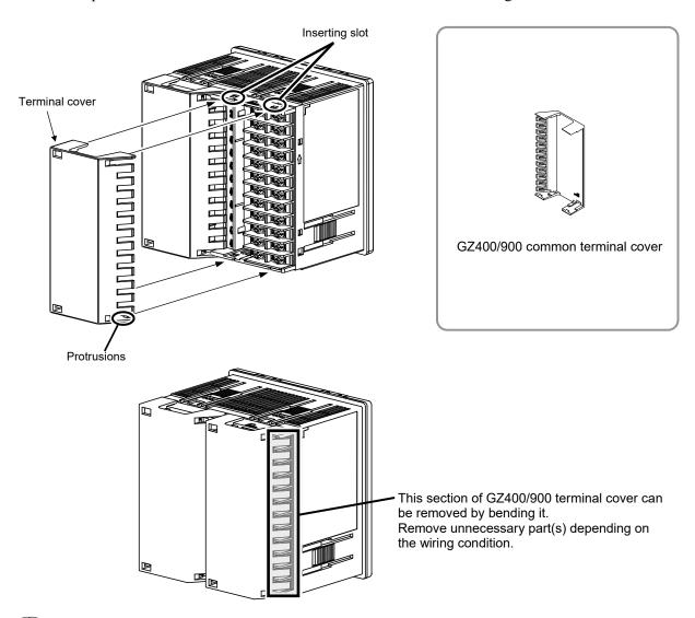
GZ900 is used in the explanatory drawing. The above mounting procedures in the example shown are the same for GZ400.
