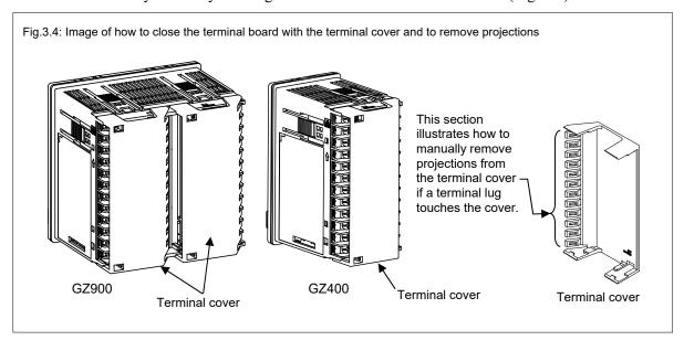
For the mounting and removing of the terminal cover, see 3.5 Handling of the Terminal Cover [Optional] (P. 3-44).
