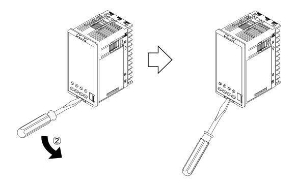
4. As the internal unit slightly comes out of the case, pull it out toward you.
