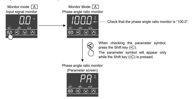
6. Check for the current value (maximum load current value) at a controller output of 100.0 %. Check for the current value at a controller output of 100.0 %. Select the CT input monitor (CT) and check the displayed current value. The value at this time is the Maximum load current value.
