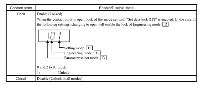
Even when this function is assigned, you can "Enable" or "Disable" the setting lock with the front key or host communication and loader communication. You can switch with "Set data lock (LE)" in Setting mode C.
