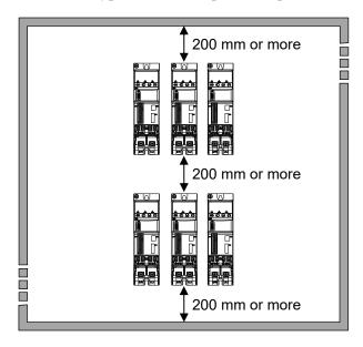
• Mount the instrument tilted within 10° from vertical (back and forth and left and right). (The figure shows 20 A/30 A types, but also observe the same angle for other models)
