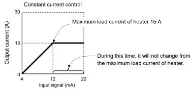
In this case, set the gradient to 50 % so that the maximum heater load current will become 15 A at an input signal of 20 mA. The gradient is valid even if internally set or set by the external gradient setter.
