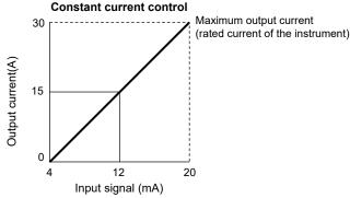
Constant current control when the rated current of the instrument is 30 A and the maximum load current of the heater is 30 A
