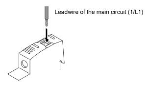
3. Tighten the screw on the front panel. Perform the wiring to the bottom side in the same way as in 1, 2 and 3.
