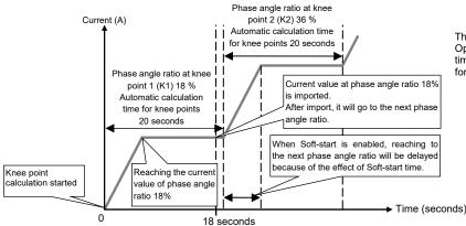
The Phase angle ratio of knee point in the Operation chart and Automatic calculation time for knee points are factory preset values for the 30A type.
