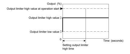
In case the Output limiter high at operation start is set at a smaller value than the Base-up set value or the Output limiter low value, priority is given to the Output limiter high at operation start.
