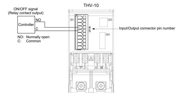
To use the contact input, the following parameters must be configured.
