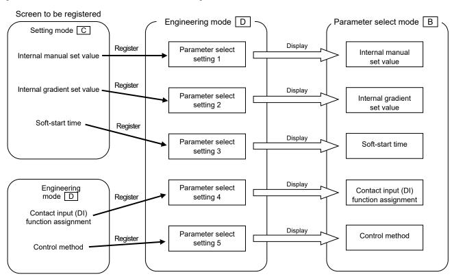
[Example] When the "Internal manual set value" screen in the Setting mode C is registered in Parameter select mode
