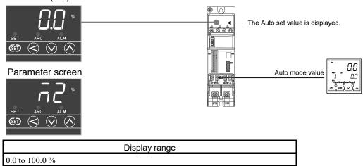
Displays the "0.0" to the Control input monitor (M2), if the controller is not connected.
