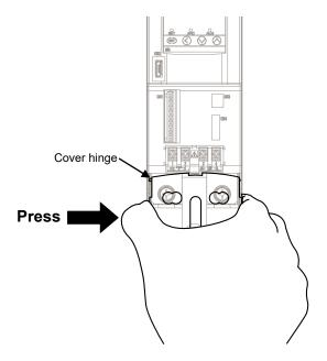
3. Once the cover hinge is out of the hole, pull the cover toward you to remove.
