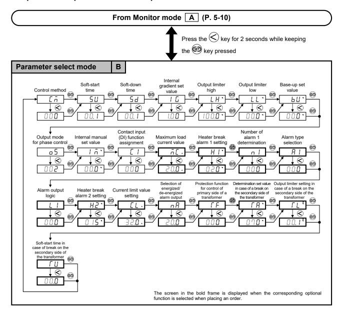
The above parameters are screens registered in Parameter select mode B by default. The screens registered in Parameter select mode B can be changed. For changing, refer to 10.4 Parameter Select Function (P. 10-12).
