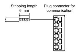
For communication connector connection, refer to 20 A/30 A/45 A/60 A/80 A/100 A THV-10 Host Communication Instruction Manual (IMR02W06-E .).
