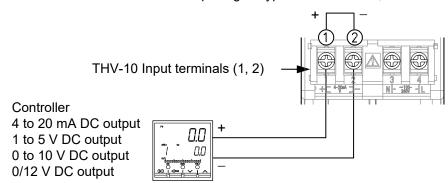
Wiring diagram of input signal
