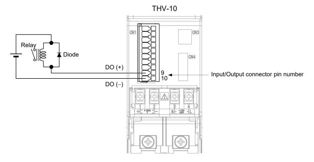
The alarm output needs to be set for the alarm type.
