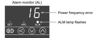
If the power frequency returns to the normal range, the alarm monitor is cleared, and the output of this instrument is also automatically released. However, if an error is determined when the instrument is turned ON, turn OFF the instrument after the power frequency returns to the normal range, and then turn it ON again.
