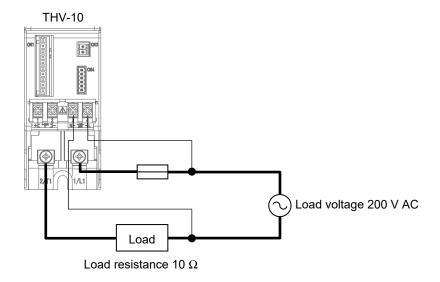
Power when the input signal is 100%
