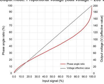
Output mode: Proportional voltage (load voltage = 200 V)
