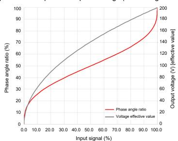
Output mode: Proportional square voltage (load voltage = 200 V)
