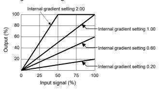
Gradient output characteristic drawing
