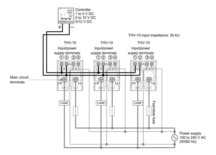
The number of THV-10 that can be connected to one temperature controller depends on the allowable load resistance of the temperature controller. For resistance of the controller, refer to specification of the temperature controller instruction manual.
