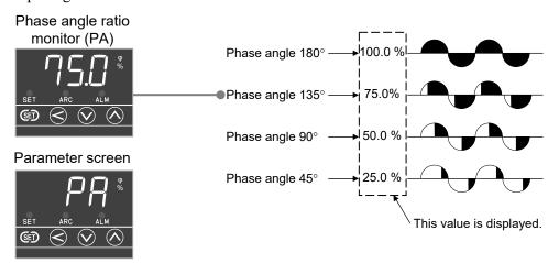
Displays 0.0% when the phase angle is  $0^{\circ}$ .
