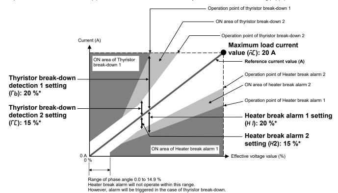
\* The alarm operation point is calculated from the deviation between the reference current value and the alarm set value. Below is an example of the calculation.
