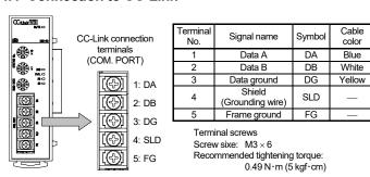
The CC-Link connecting terminal cannot do on-line installation or dismount for terminal block of dismount impossibility. The device cannot be replaced unless the link is set off-line. In addition, FG (frame ground) terminal of terminal number 5 is FG in a CC-Link function, and it is not FG of instrument all.
