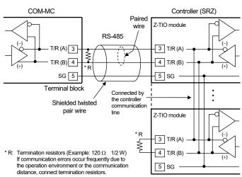
Up to 16 Z-TIO modules can be connected.
