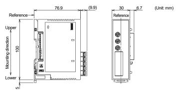
Allowable tilt angle is  $\pm 90^{\circ}$ , back and force, right and left from the reference.
