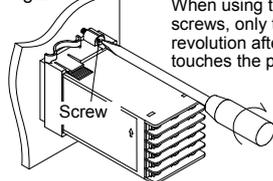
When using the mounting screws, only turn one full revolution after the screw touches the panel.
