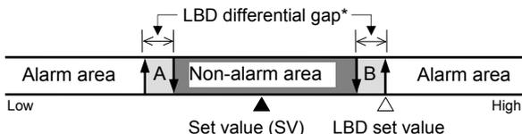
A: During temperature rise: Alarm area      B: During temperature rise: Non-alarm area
