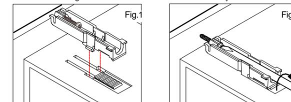
When the instrument is mounted, always secure with two mounting brackets so that upper and lower mounting brackets are positioned diagonally.
