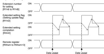
Regardless of the number of occupied stations and the extended cyclic, the above processing is also necessary if the Set value (SV) assigned to the Remote register (RWw) as a fixed value is changed
