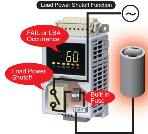
\* Internal fuse must be replaced by an authorized personnel.
