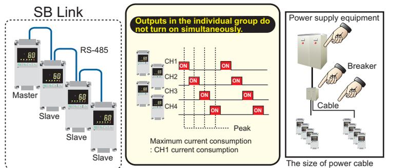
The size of power cable and power supply equipment can be minimized.
