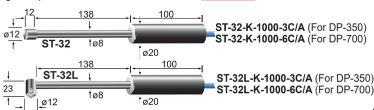
For semi-solid, viscous material and liquid Unit:mm
