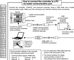
Parity bit: None Stop bit: 1 Communication port of host comput USB port: Based on USB Ver. 2.0
