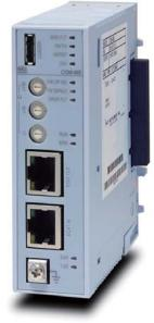
COM-ME-3 can be used to connect our SRZ series, FZ series, and GZ series to the EnterCAT network.
